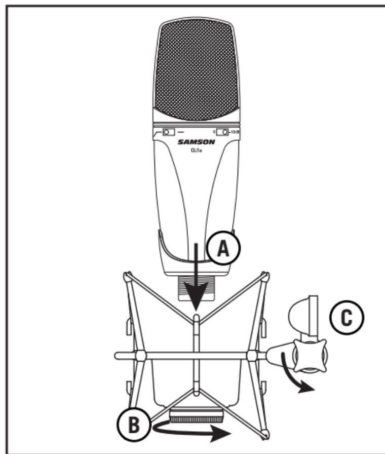
For additional isolation the CL8a can be fitted on the optional SP01 spider shockmount to isolate the microphone from vibrations and mechanical noises transmitted through the mic stand. Follow the steps below to mount the CL8a to the SP01.
