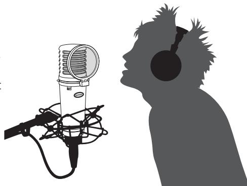
microphone center line towards their mouth. If some consonants such as 'P' and 'S' seem to jump up in level, rotate the microphone a little bit away from the artist so that sound arrives at the microphone slightly off-center. It is preferable to prevent these peaks through the use of the MPF1 external pop filter. If recording a group of singers, ensure that they position themselves around the front of the microphone close to one another.
