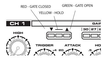
To get the gate to operate fast, smoothly and predictably use the ATTACK, HOLD and RELEASE controls to contour the shape.
