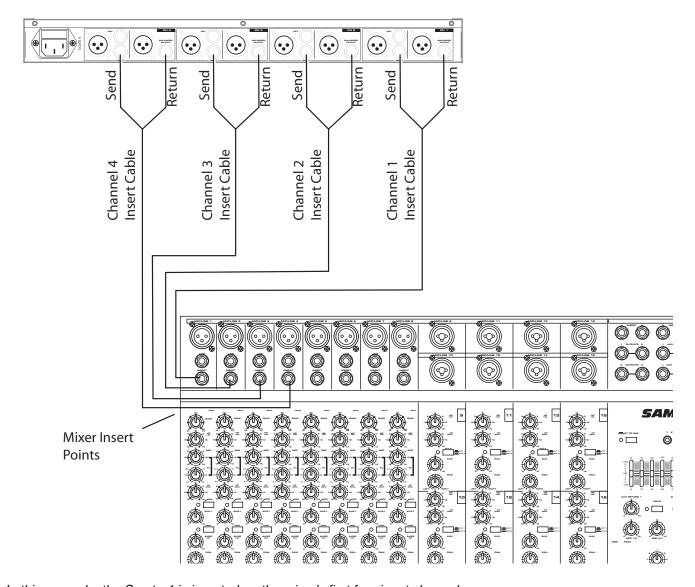
In this example, the S gate 4 is inserted on the mixer's first four input channels.
