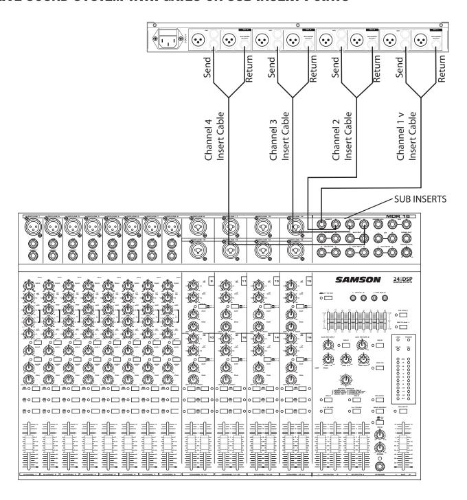
In this example, the S gate 4 channels are connected to the mixer's bus 1-4 inserts points.
