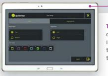
Text Overlay. Configure on-screen display of text, including variables like zoom, tilt and GPS coordinates. Modify text color and position.
