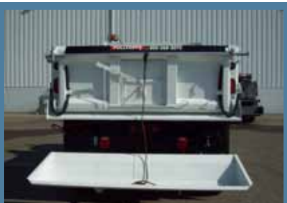
Shoveling Apron for Asphalt, Sand or Other Materials
