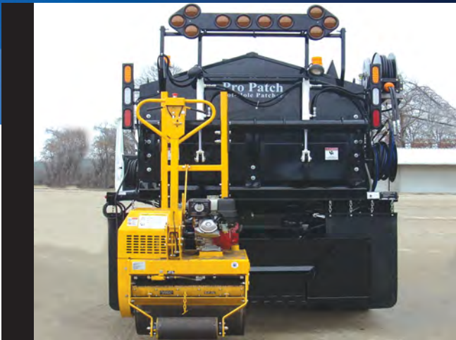
Dump body (4 or 5 cubic yards) LP or CNG gas heating system. 80 or 120 Emulsion tank. Class 50, 40 ton hoist tack spray and hydraulic tools.
