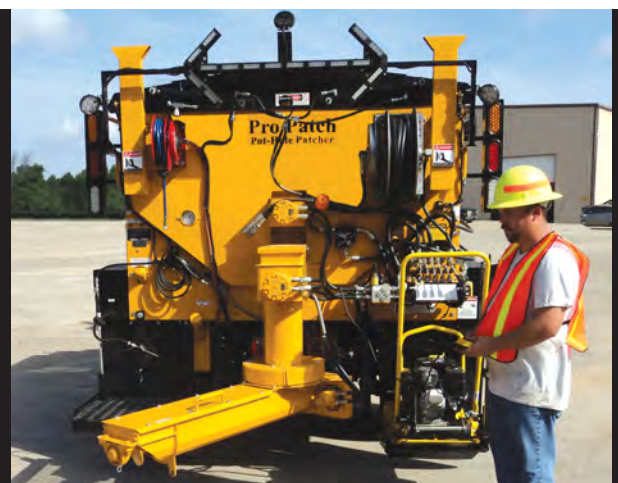
Asphalt Spreader Used to repair large cut and long trenches. Available in manual or remote control.
