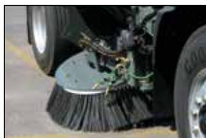
In-cab side broom tilt and extended reach
