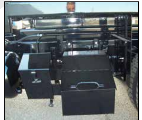
Sand box carries base material for deeper potholes and a solvent dip tank to clean tools before and after patching.
