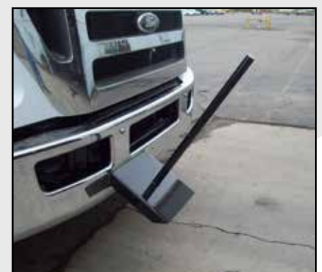
Bumper mounted Cone Holders save space and increase visibility.
