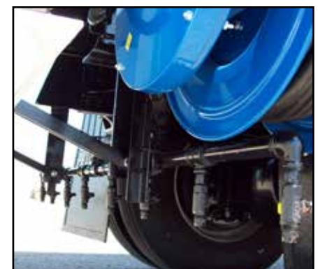
Spray bars allow your pothole patcher to double as a liquid asphalt distributor when necessary.
