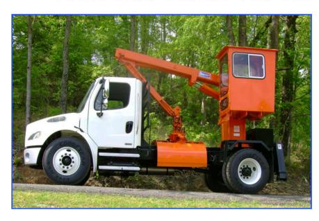
The Shuttle loader can be equipped with either a seat mount or an enclosed cab with sliding side windows. Air conditioning and heat are also available with the cab unit.
