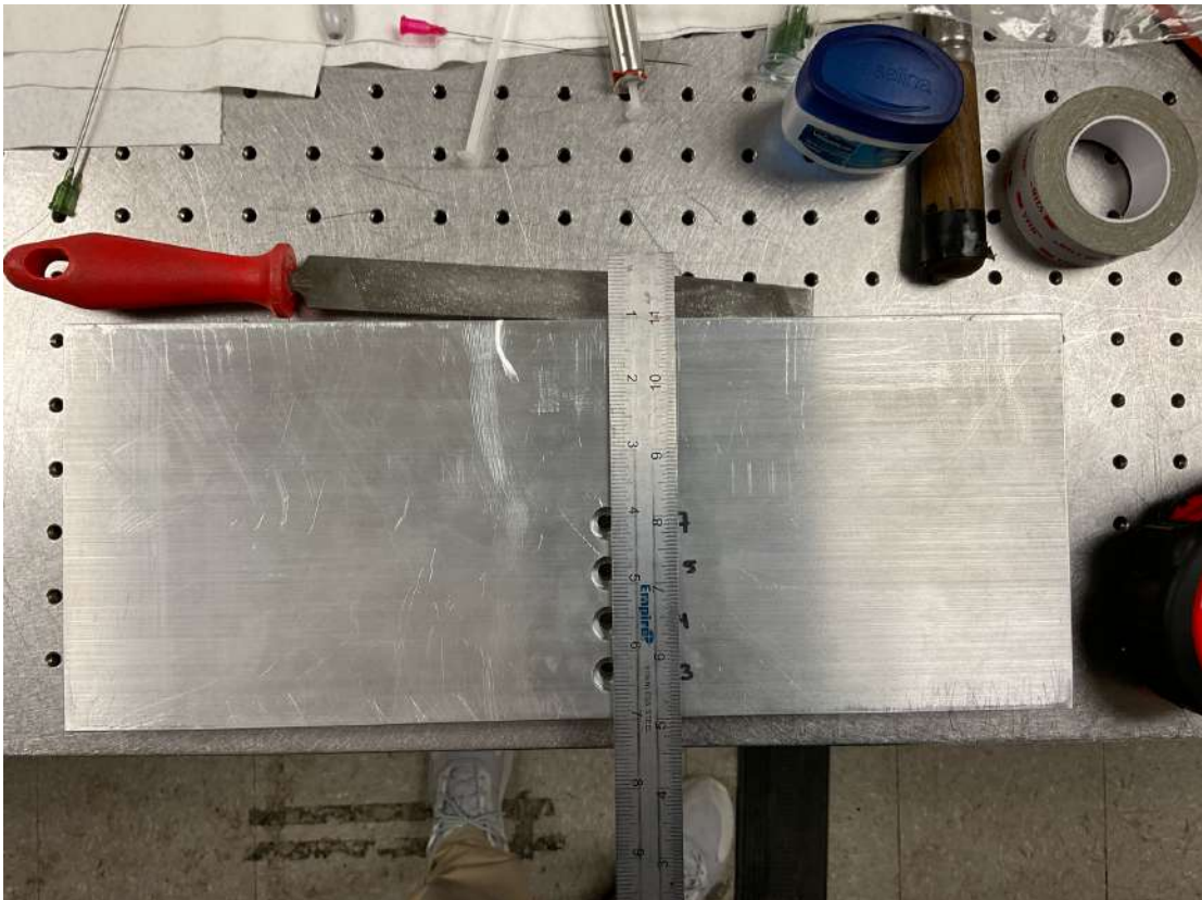
Figure A.3.2: Vertical array of pressure measurement taps on the metal window
