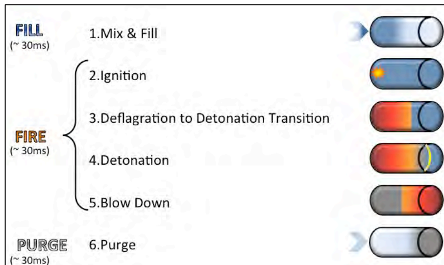
Figure 2. PDE combustion process
