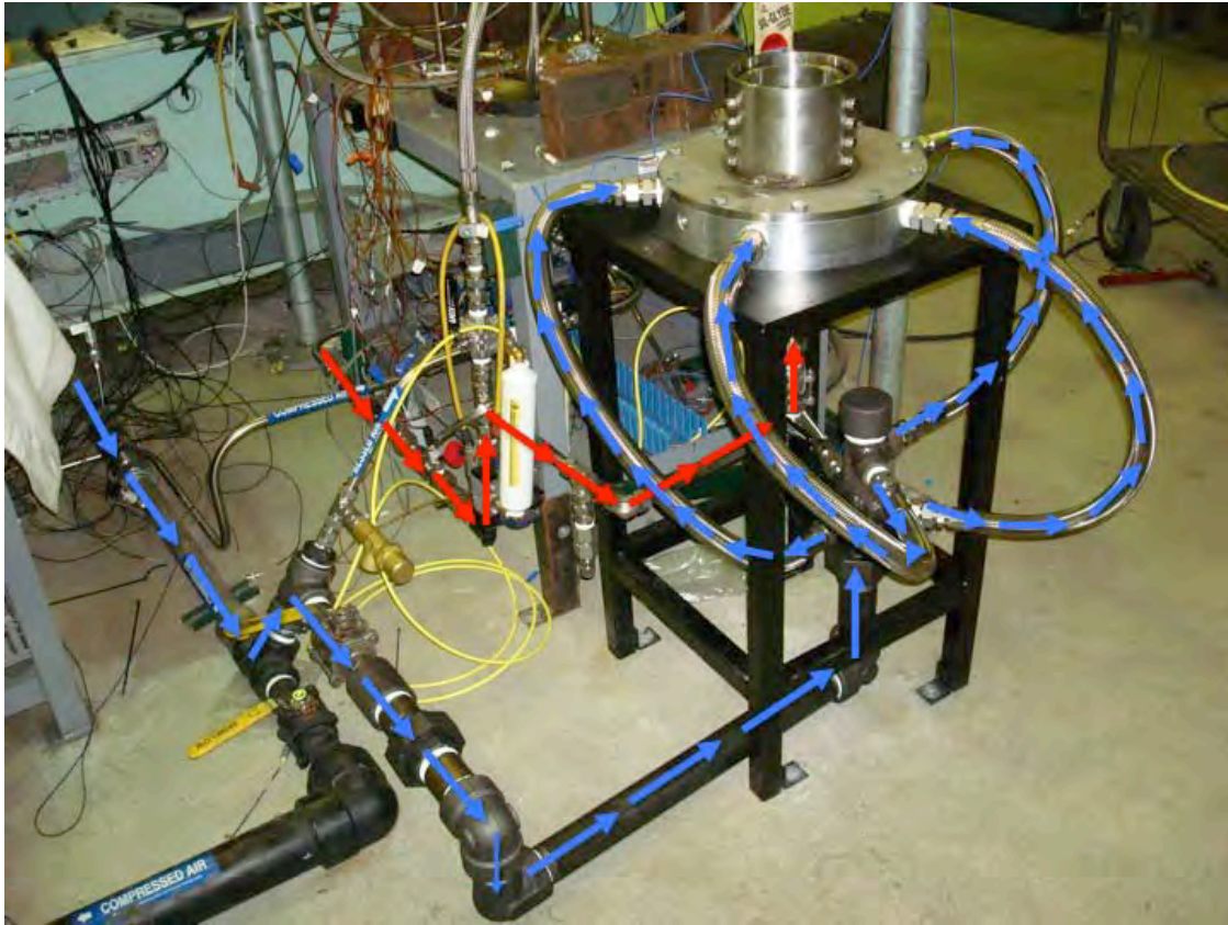
Figure 19. Highlighted oxidizer and fuel supply lines with flow path highlighted
