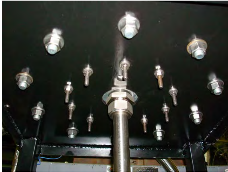
Figure 14. Bottom of RDE test stand showing attachment and fuel supply line
