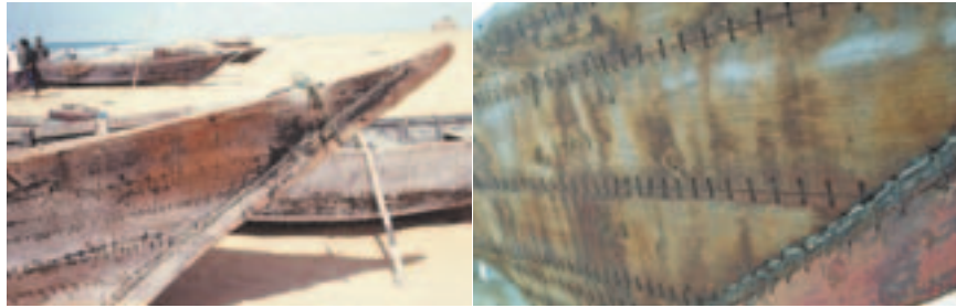
Sewn ships are rarely seen today. This example was on a remote beach in al-Mahra province, eastern Yemen in 1992. The close-up of the timber stitching is of an Omani ship.
