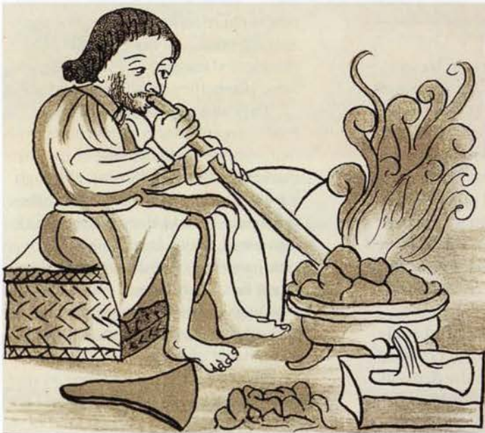
Sahagun's Florentine Codex pictures an Aztec metalworker plying his craft with a very simple but effective apparatus. Molten copper pours from the crucible into a mold to form an axe head.
