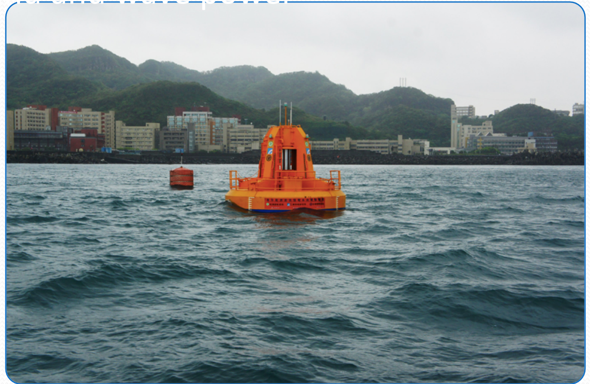
Sea trial of a 20 KW wave power generator developed by CSBC
