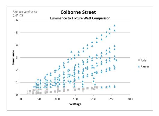
Of the fixtures analyzed, the lowest energy consuming fixture that met the light performance criteria had an energy consumption of 36 watts. While some fixtures with lower energy consumption were able to provide this level of average luminance, they failed due to unacceptable uniformity.
