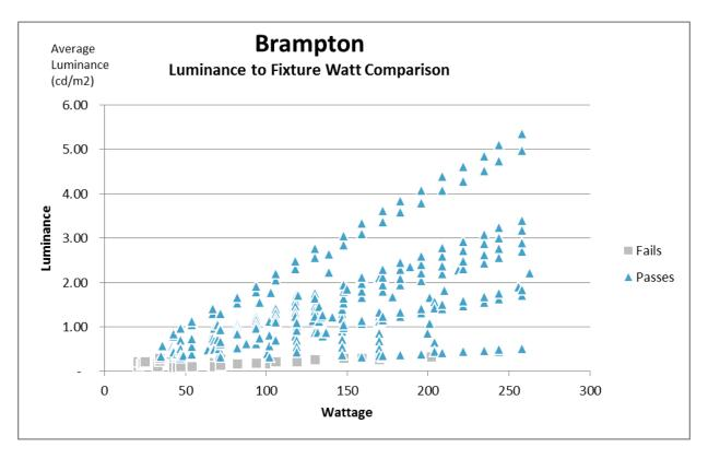
Of the fixtures analyzed, the lowest energy consuming fixture that met the light performance criteria had an energy consumption of 35 watts. While some fixtures with lower energy consumption were able to provide this level of average luminance, they failed due to unacceptable uniformity.
