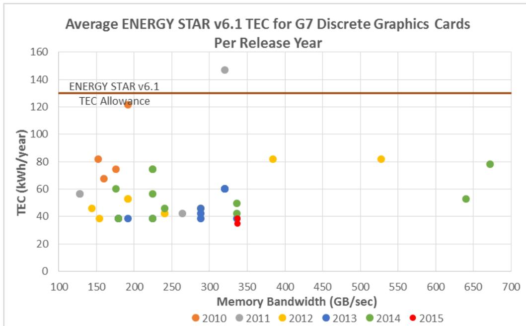
Figure 25 – Average ENERGY STAR v6.1 based TEC of High End Discrete GPUs per Year of Release Compared to the ENERGY STAR v6.1 allowances
