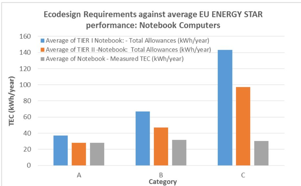
Figure 2 – Average TEC for Notebook Computers in the EU ENERGY STAR database over time compared to the EU Ecodesign Requirements
