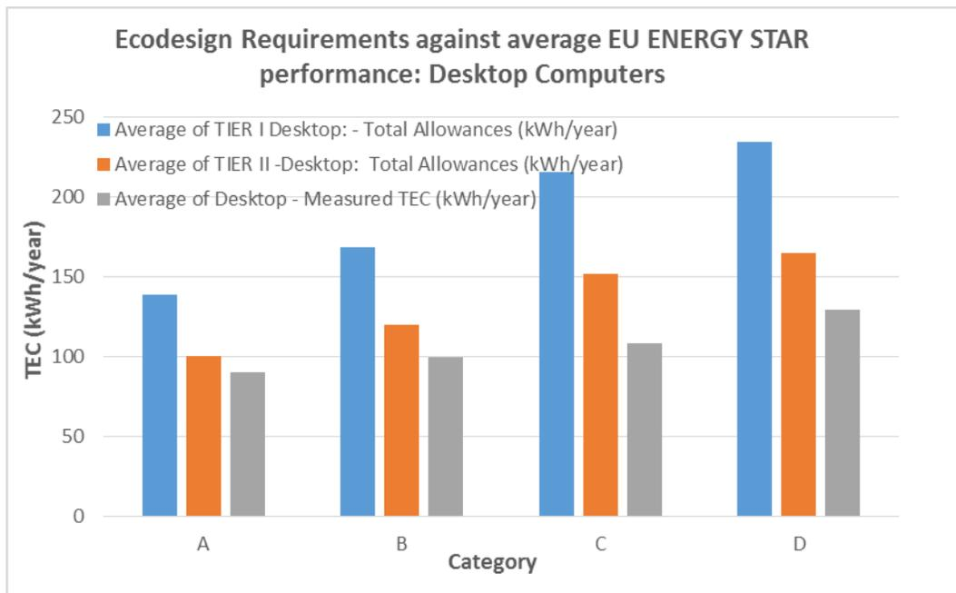
Figure 9 – Average TEC for Desktop Computers in the EU ENERGY STAR database over time compared to the EU Ecodesign Requirements
