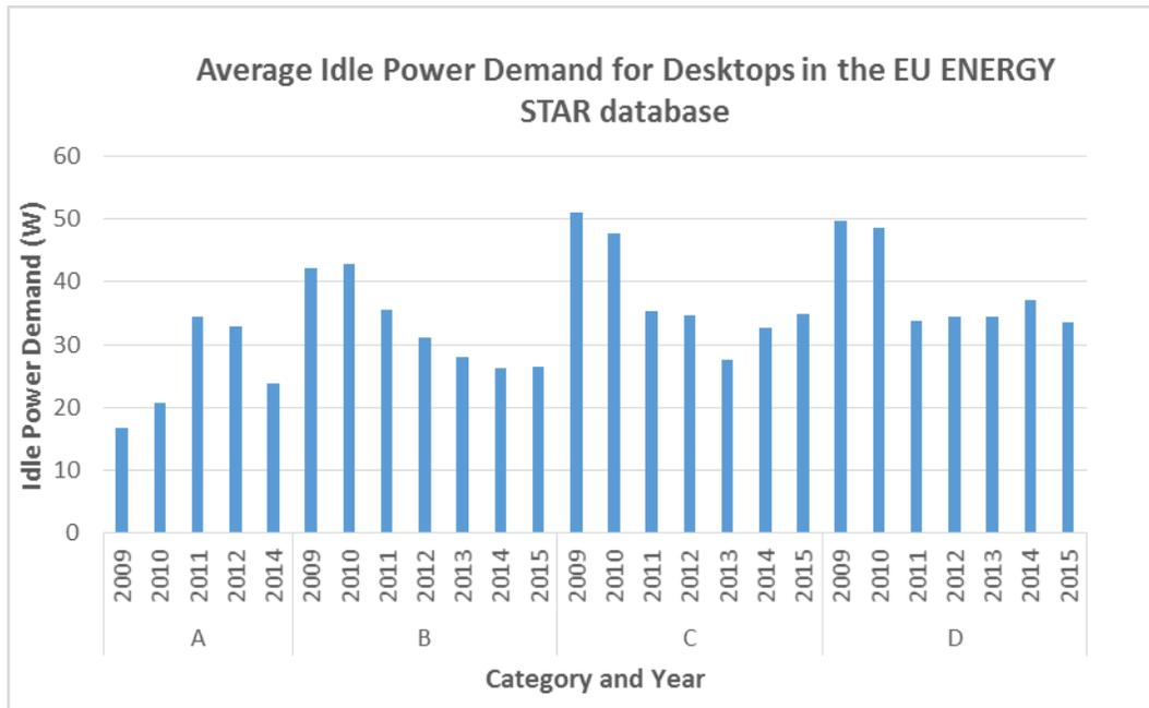
Figure 1 – Average ENERGY STAR v5.1 based Idle Mode Power Demand of desktop computers in the EU ENERGY STAR database
