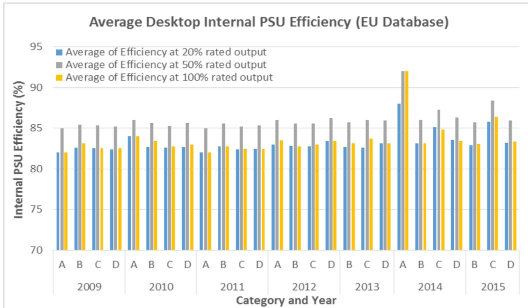
Figure 30 – Average Internal PSU Efficiency at different loading points for Desktop Computers in the EU ENERGY STAR database
