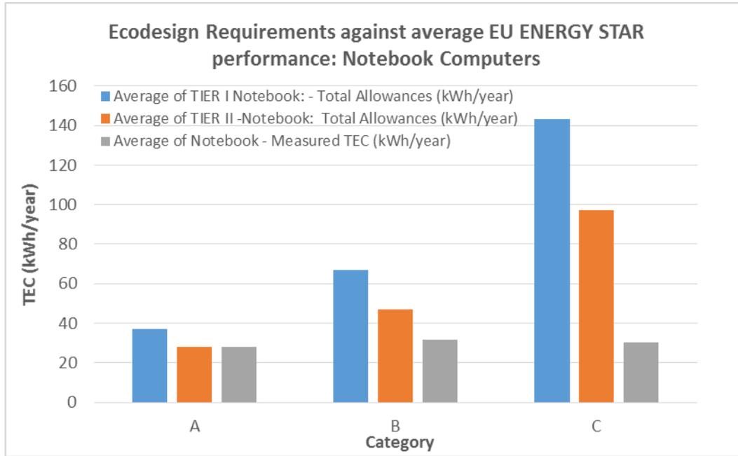
Figure 10 – Average TEC for Notebook Computers in the EU ENERGY STAR database over time compared to the EU Ecodesign Requirements
