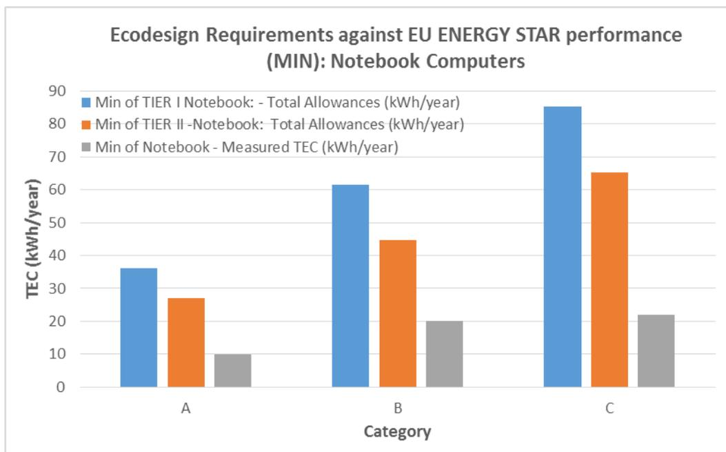
Figure 12 – Minimum TEC for Notebook Computers in the EU ENERGY STAR database over time compared to the EU Ecodesign Requirements
