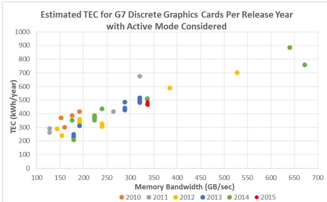
Figure 27 – Average TEC of High End Discrete GPUs per Year of Release Compared with Active Mode Considered
