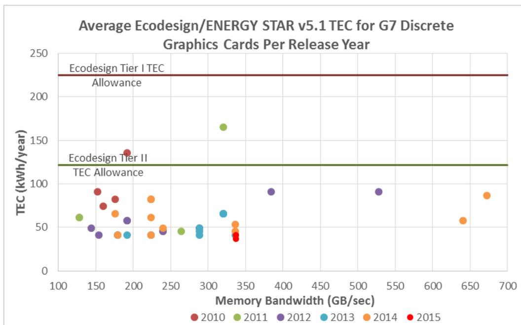
Figure 5 – Average TEC of High End Discrete GPUs per Year of Release Compared to the EU Ecodesign Allowances
