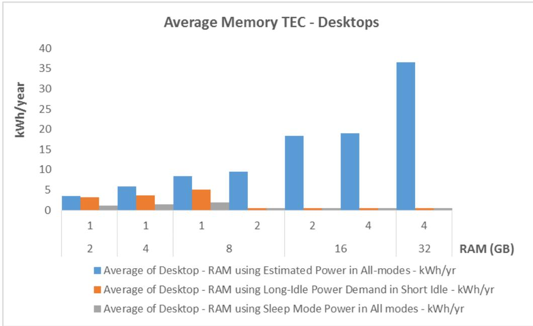
Figure 40 – Average Desktop based TEC for Sample RAM Modules
