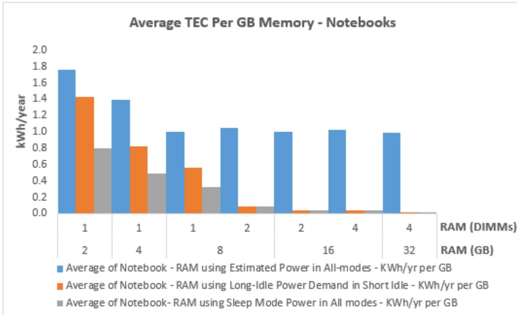
Figure 39 – Average Notebook based TEC per GB of RAM for Sample RAM Modules
