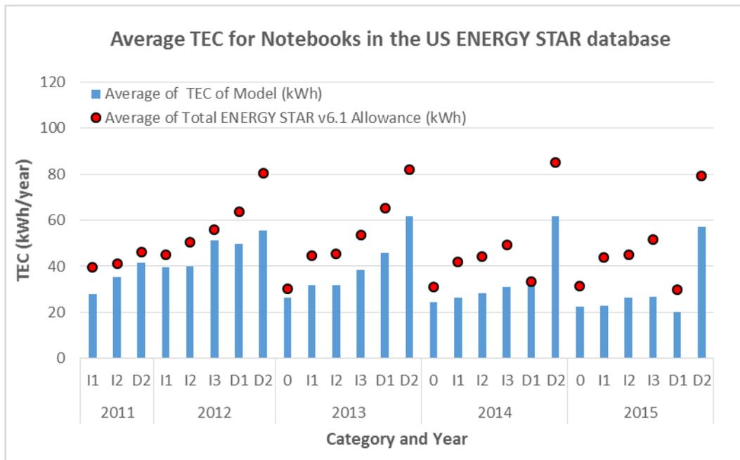
Figure 4 – Average TEC for Notebook Computers in the US ENERGY STAR database based on year first placed on the market against average ENERGY STAR v6.1 TEC allowance
