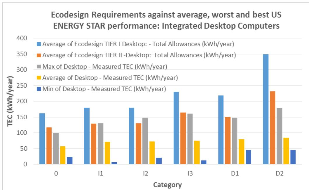
Figure 20 – Average EU Ecodesign Regulation TEC requirements for Integrated Desktop Computers in the US ENERGY STAR database against average, maximum and minimum TEC values
