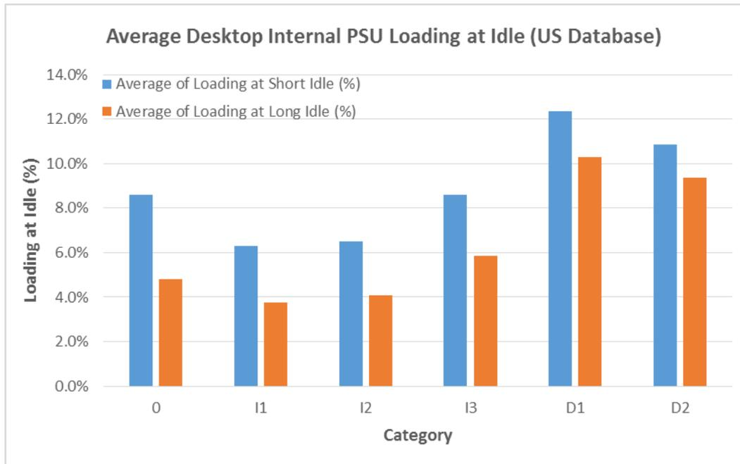
Figure 35 – Average Internal PSU Loading at Short and Long Idle for Desktop Computers in the US ENERGY STAR database
