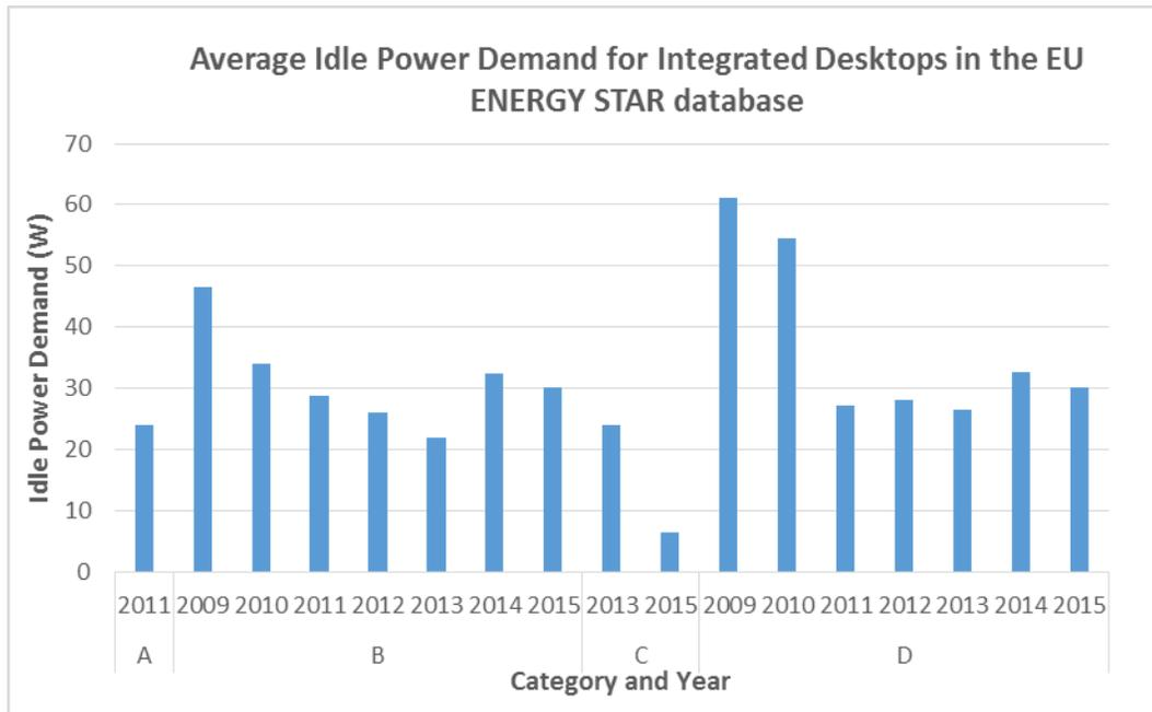
Figure 2 – Average ENERGY STAR v5.1 based Idle Mode Power Demand of integrated desktop computers in the EU ENERGY STAR database
