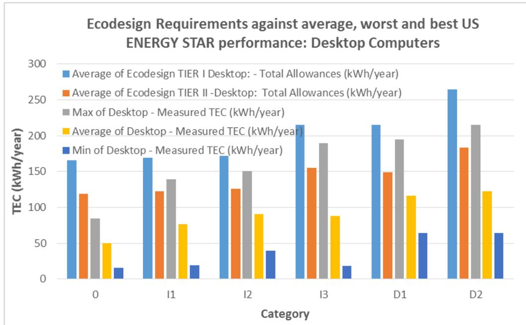
Figure 19 – Average EU Ecodesign Regulation TEC requirements for Desktop Computers in the US ENERGY STAR database against average, maximum and minimum TEC values
