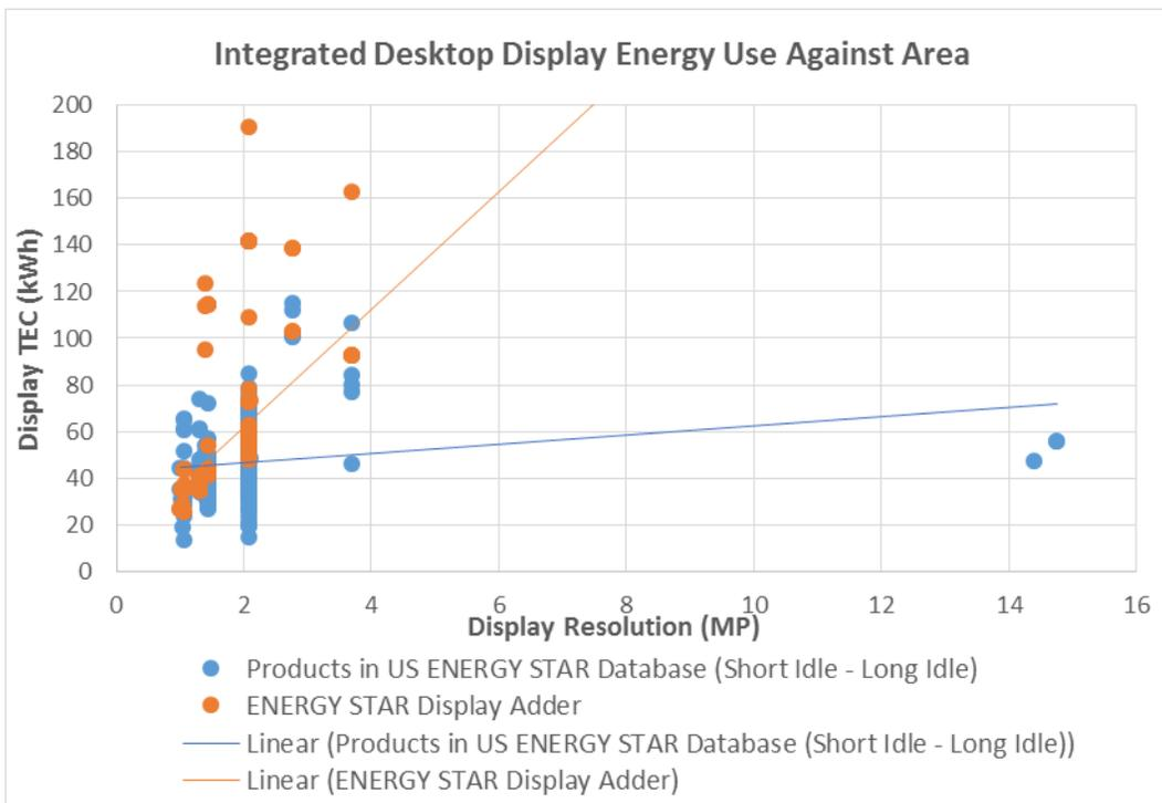
Figure 37 – Estimated ENERGY STAR v6.1 TEC of Displays and Allowances in Integrated Desktop Computers Listed in the US ENERGY STAR database (May 2015) against Resolution
