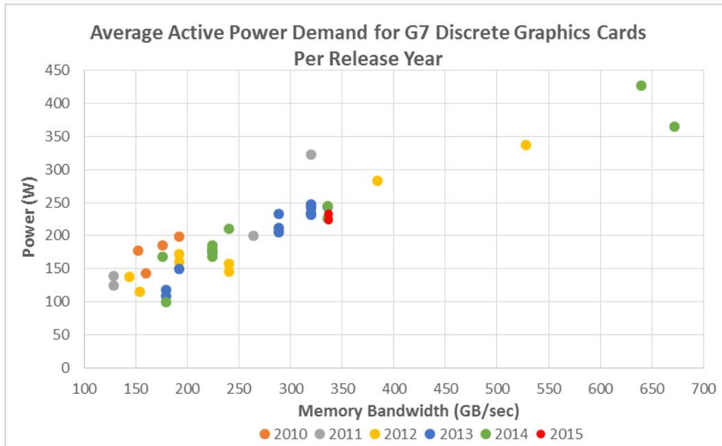
Figure 26 – Average Active Mode Power Demand in High End Discrete GPUs per Year of Release
