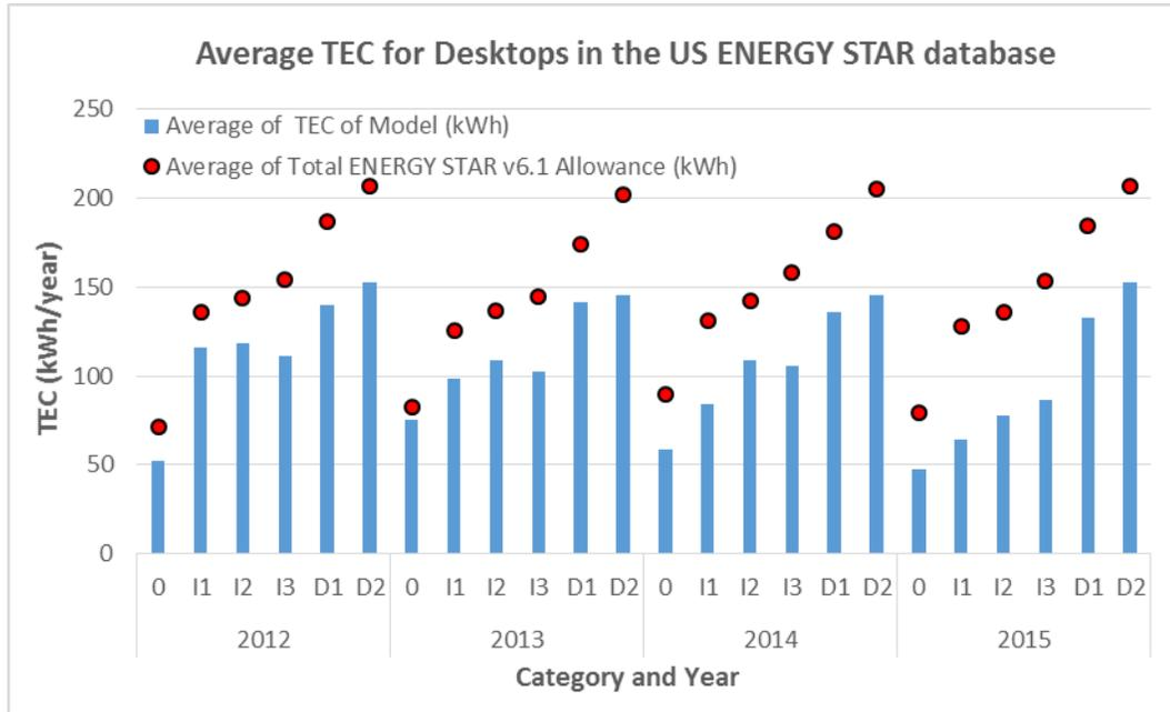
Figure 3 – Average TEC for Desktop Computers in the US ENERGY STAR database based on year first placed on the market against average ENERGY STAR v6.1 TEC allowance
