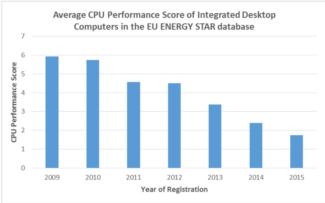
Figure 5 – Average CPU Performance Score for Integrated Desktop Computers in the EU ENERGY STAR database over time
