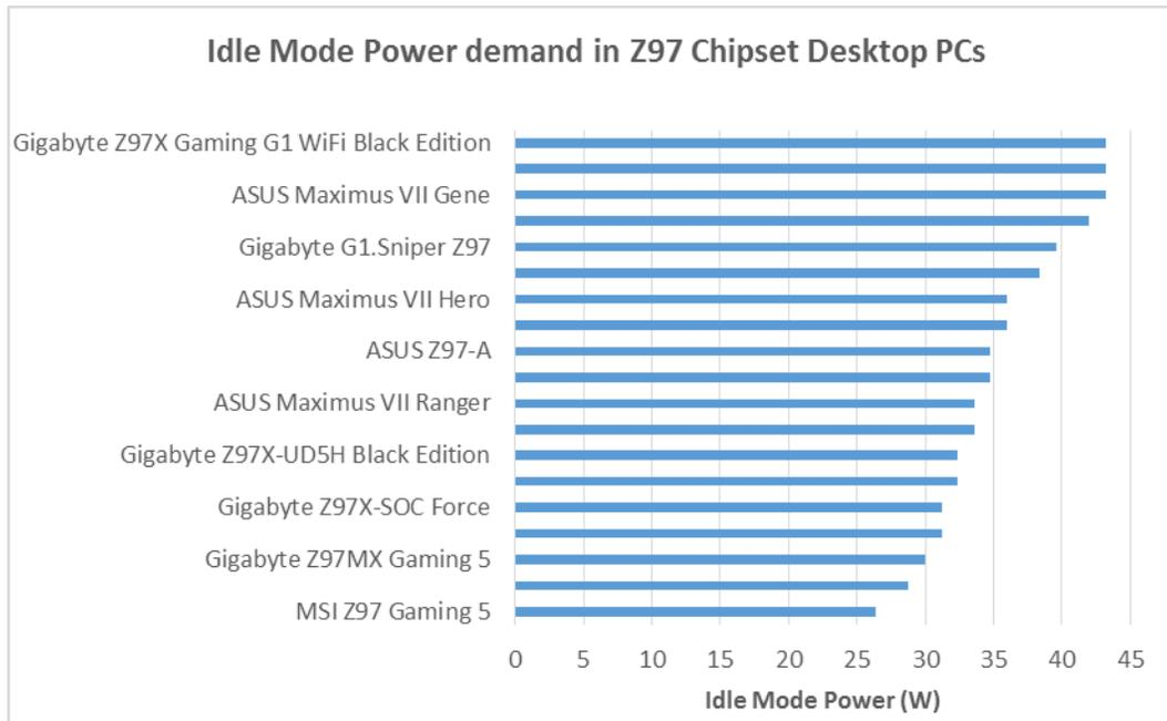
Figure 22 – Idle Mode Power demand of Z97 Chipset Motherboards<sup>7</sup>
