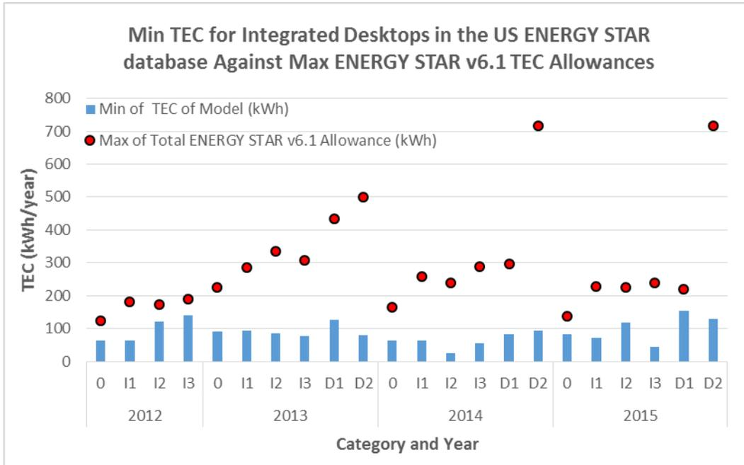
Figure 17 – Minimum TEC found for Integrated Desktop Computers in the US ENERGY STAR database based on year first placed on the market against the maximum ENERGY STAR v6.1 TEC allowance found
