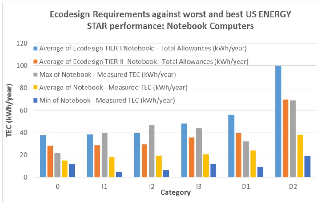
Figure 21 – Average EU Ecodesign Regulation TEC requirements for Notebook Computers in the US ENERGY STAR database against average, maximum and minimum TEC values
