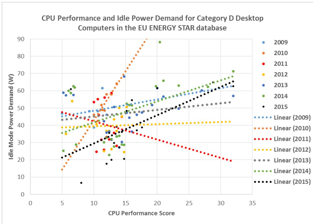
Figure 7 – Average Idle Mode Power Demand for Category D Desktop Computers in the EU ENERGY STAR database against CPU Performance
