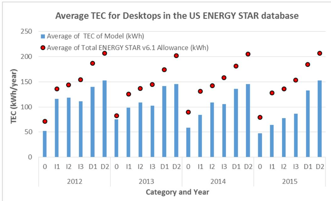
Figure 13 – Average TEC for Desktop Computers in the US ENERGY STAR database based on year first placed on the market against average ENERGY STAR v6.1 TEC allowance
