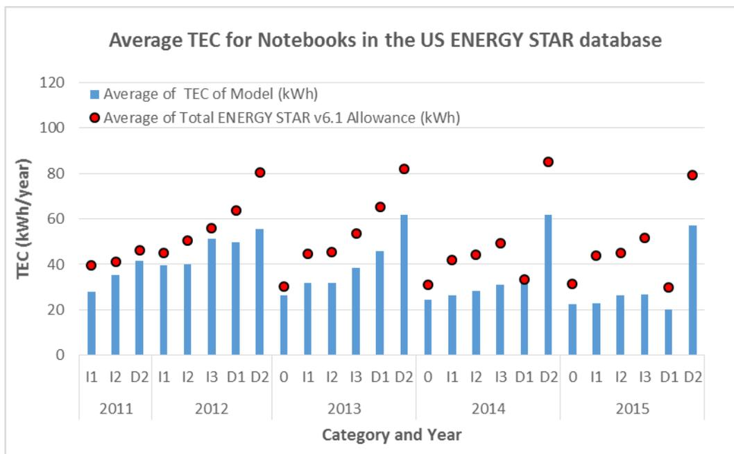
Figure 15 – Average TEC for Notebook Computers in the US ENERGY STAR database based on year first placed on the market against average ENERGY STAR v6.1 TEC allowance
