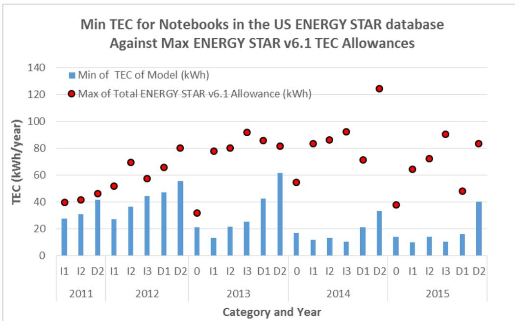
Figure 18 – Minimum TEC found for Notebook Computers in the US ENERGY STAR database based on year first placed on the market against the maximum ENERGY STAR v6.1 TEC allowance found
