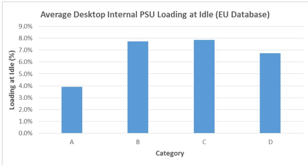
Figure 34 – Average Internal PSU Loading at Idle for Desktop Computers in the EU ENERGY STAR database
