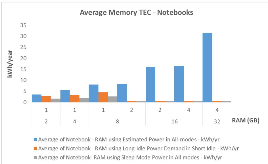
Figure 41 – Average Notebook based TEC for Sample RAM Modules
