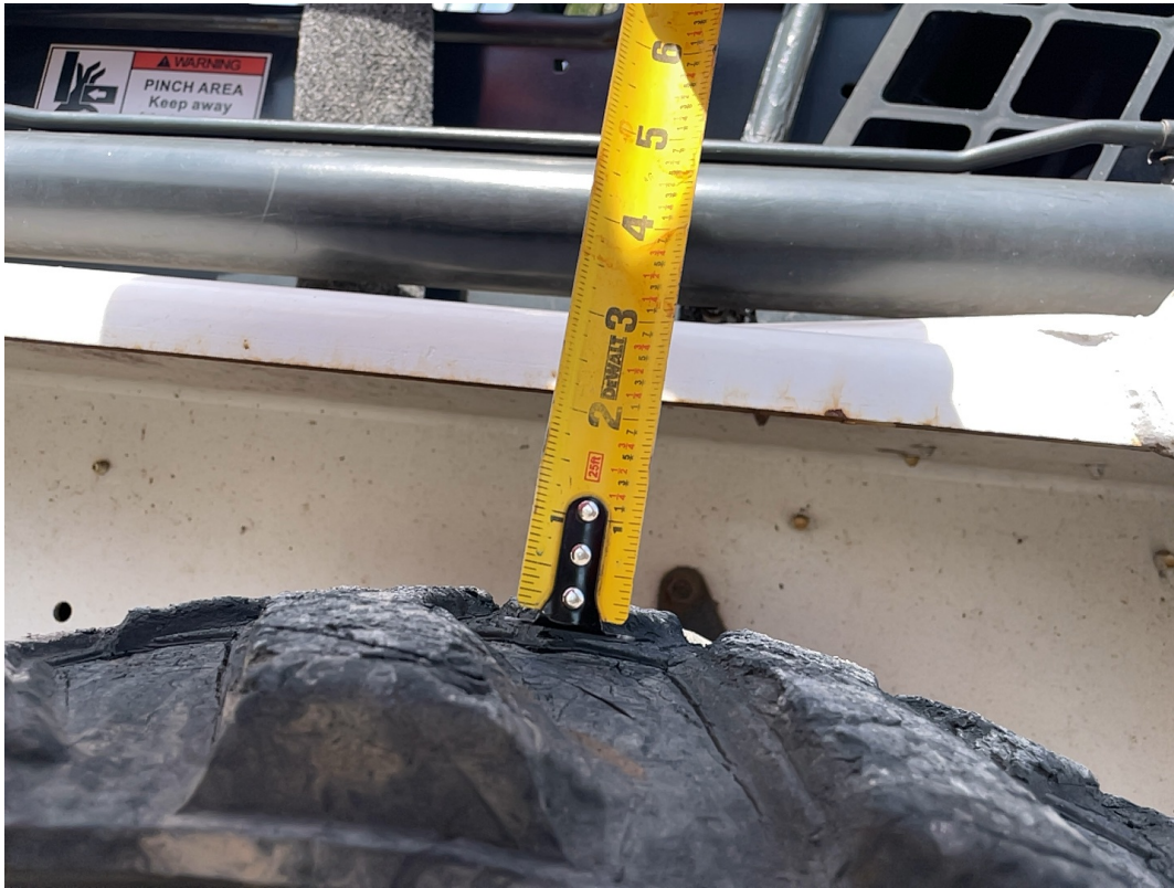
Rear Left Tire Tread Depth Measurement / 05-15-2024
