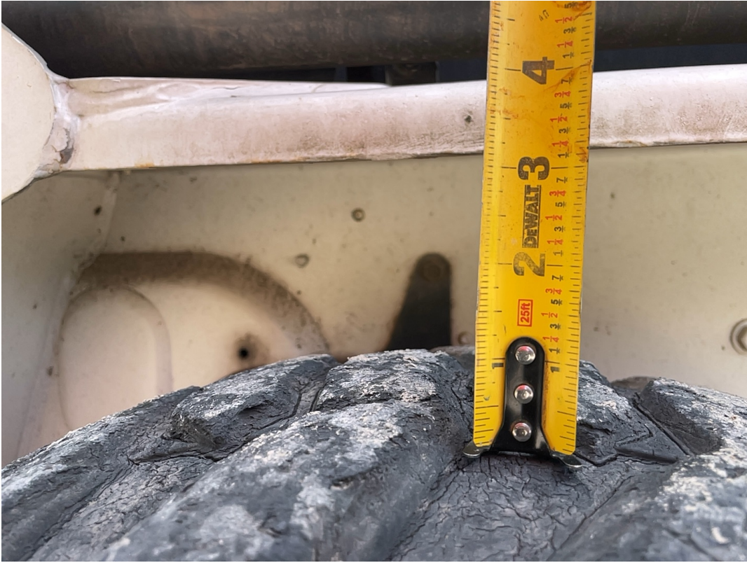
Rear Right Tire Tread Depth Measurement / 05-15-2024
