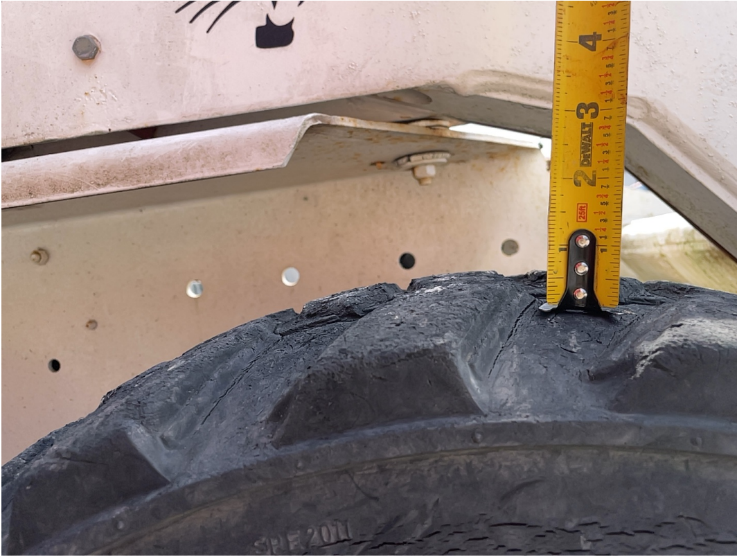
Front Right Tire Tread Depth Measurement / 05-15-2024
