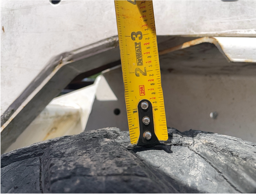
Front Left Tire Tread Depth Measurement / 05-15-2024
