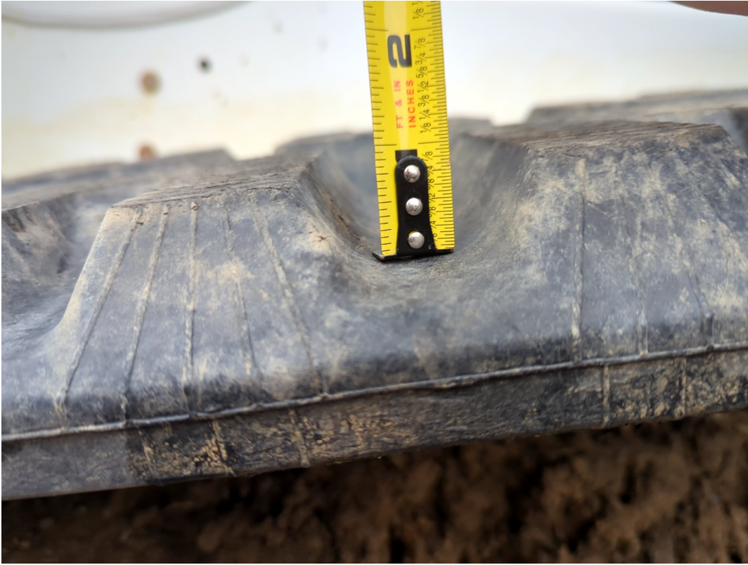
Left Track Tread Depth Measurement / 03-05-2024
