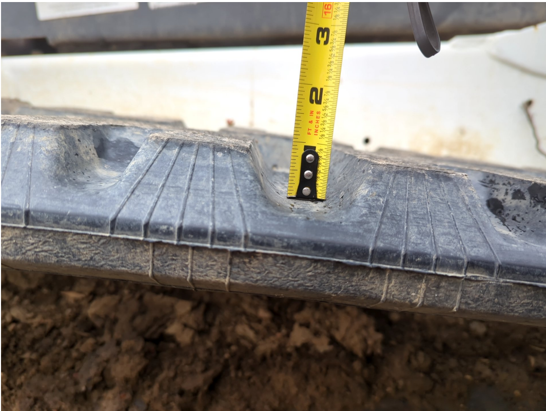
Right Track Tread Depth Measurement / 03-05-2024
