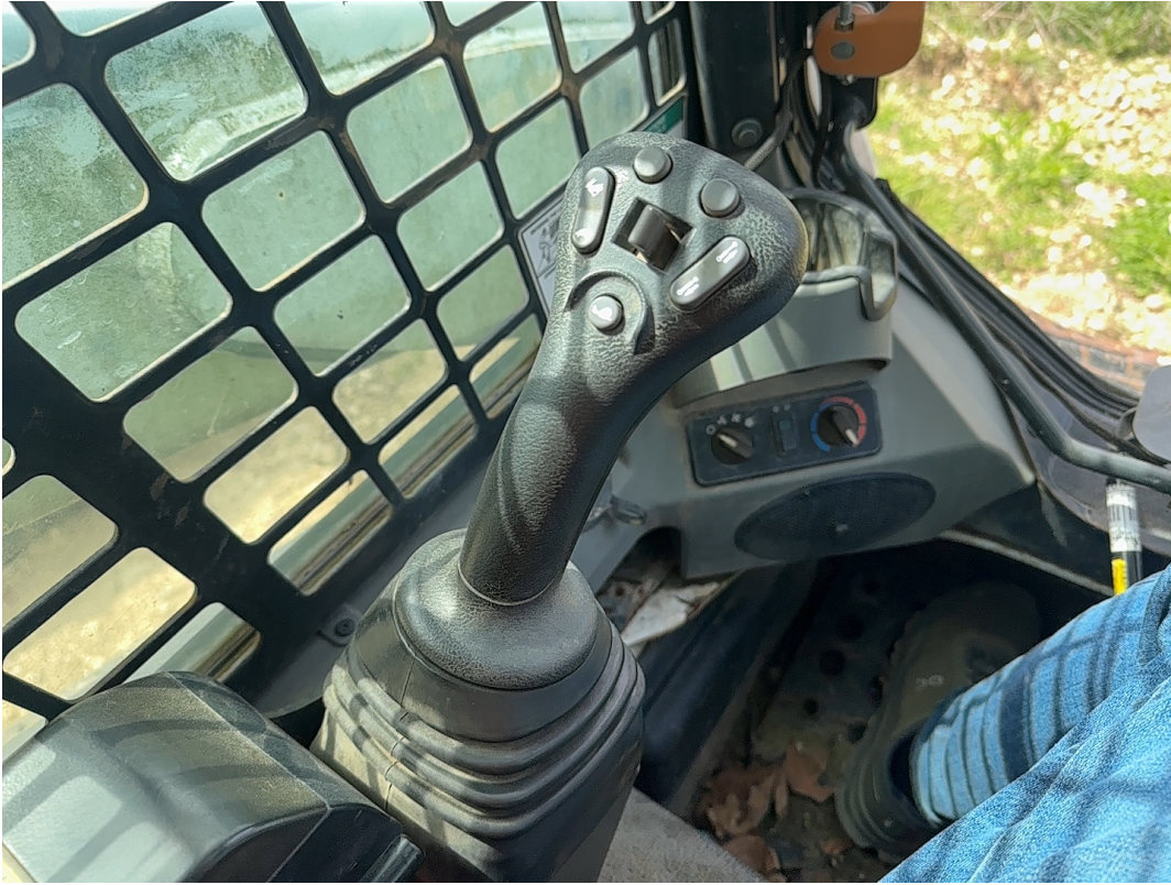
Switches and Controls / Travel Control / 04-26-2024
