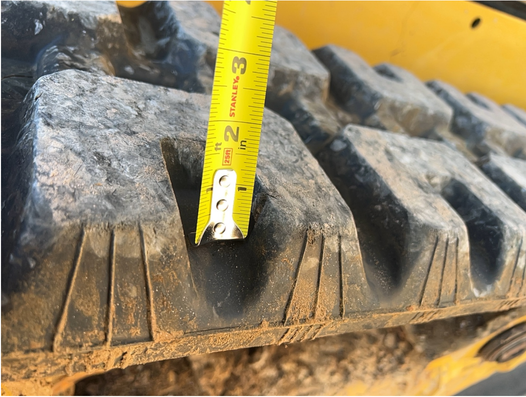
Right Track Tread Depth Measurement / 03-19-2024
