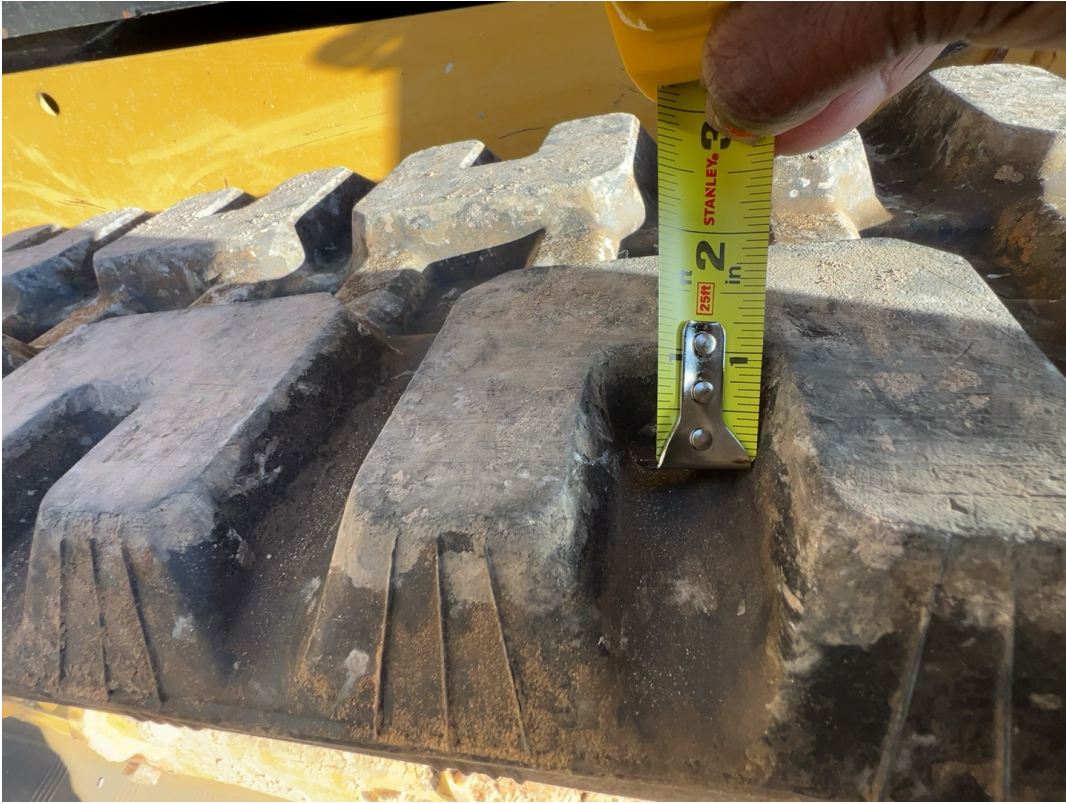
Left Track Tread Depth Measurement / 03-19-2024
