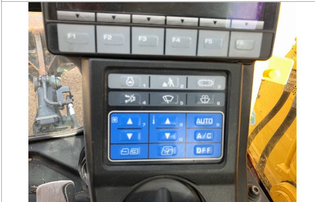
A/C / Switches and Controls
