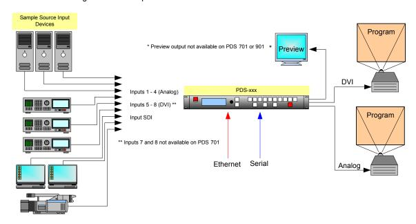
Figure 3-1. PDS System Diagram (sample)
