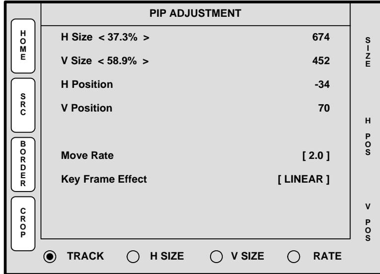
Figure 4-31. PIP Adjustment Menu (sample)
