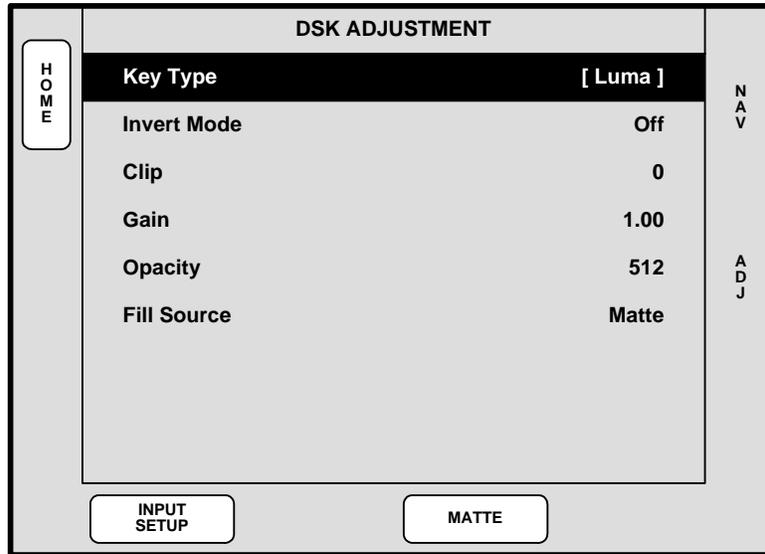
Figure 4-48. DSK Adjustment Menu (sample)
