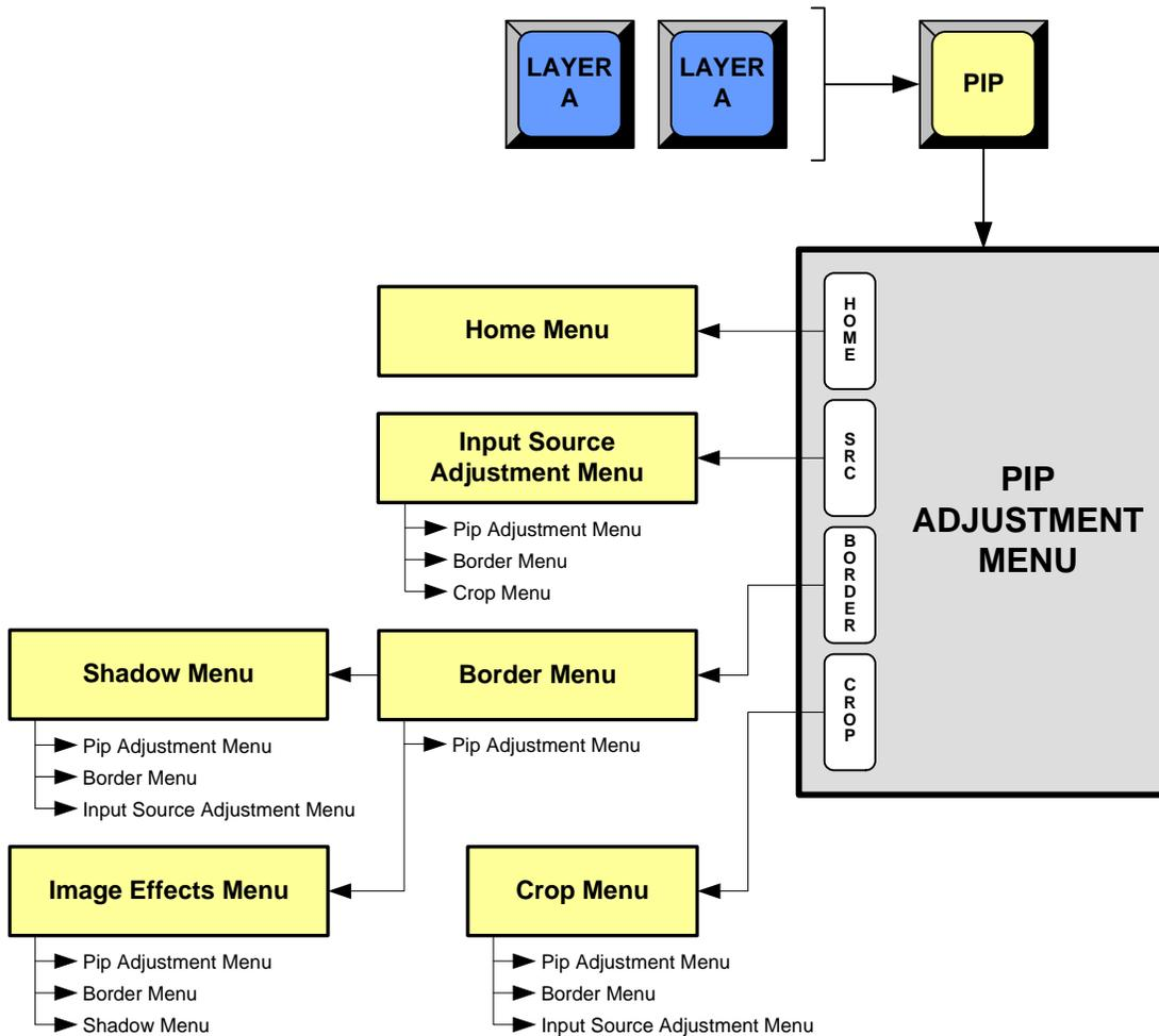
Figure 4-30. PIP Adjustment Menu Tree
