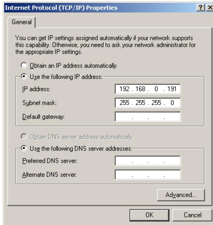
**Figure C-7.** Internet Protocol (TCP/IP) Properties Dialog (sample)
