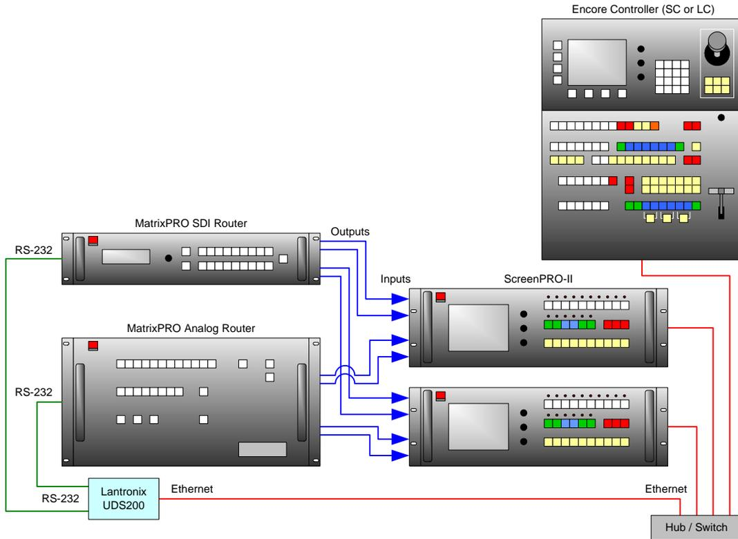
**Figure D-2.** ScreenPRO-II Units using External Serial Controlled Routers
