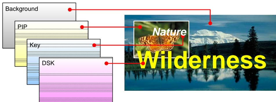
Figure 1-2. Layer Illustration — Background, Mixer and DSK
