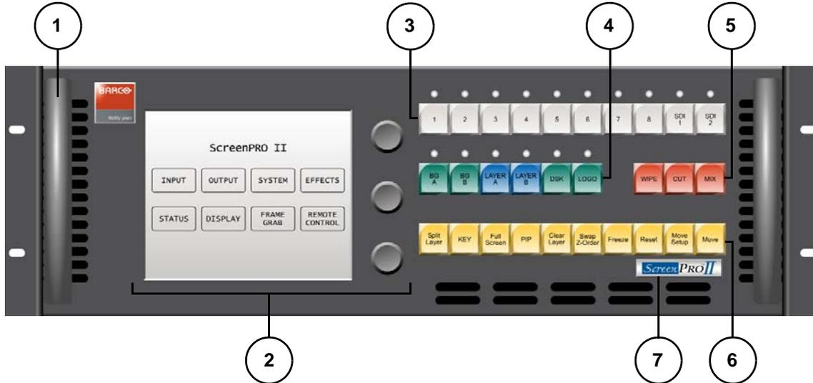
Figure 2-1. ScreenPRO-II Front Panel
