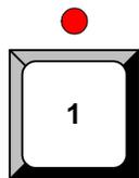
Press a button in the section to assign the source to the blinking “mixer” button in the **Layer Control Section**. When the button is lit and blinking, the source is on Preview, and is active for manipulation as the PIP or key source on that layer.
