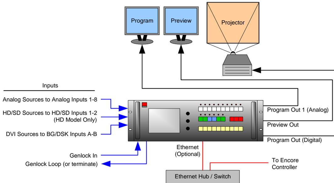
**Figure 3-1.** Block Diagram, Basic ScreenPRO-II System
