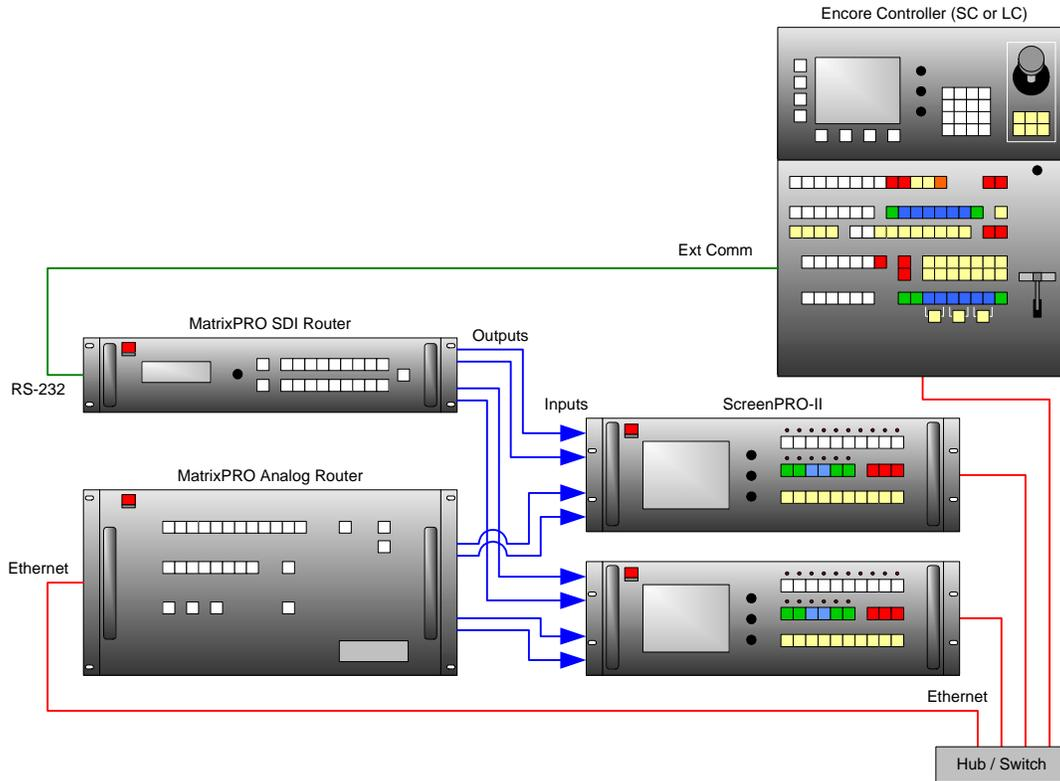
**Figure D-4.** ScreenPRO-II Units using External Serial and Ethernet Controlled Routers
