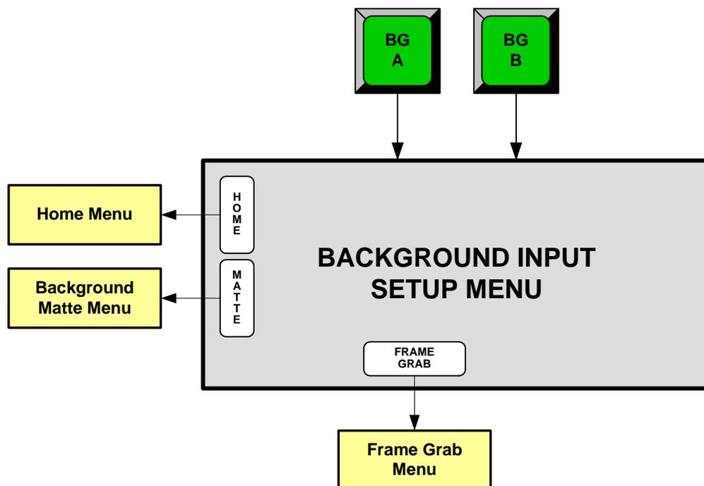
**Figure 4-42.** Background Input Setup Menu Tree
