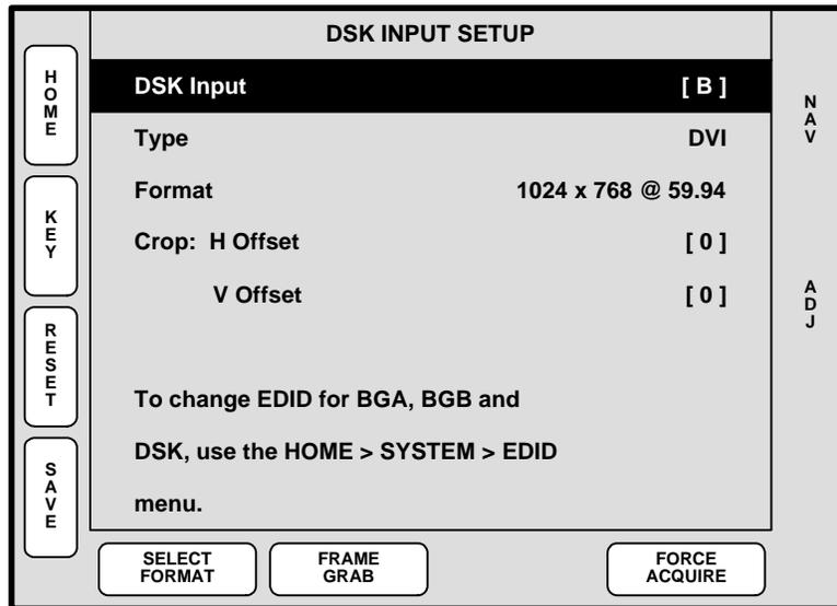
Figure 4-49. DSK Input Setup Menu (sample)
