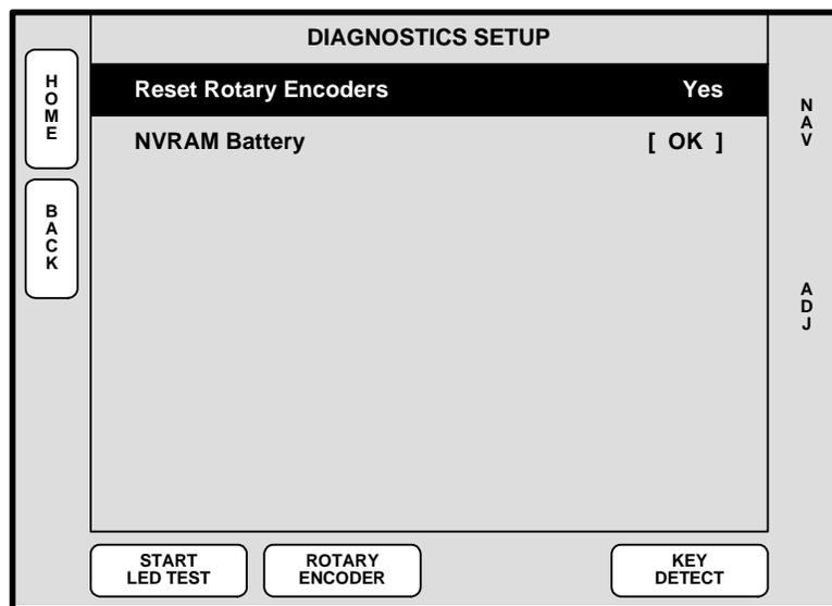
Figure 4-18. Diagnostics Setup Menu (sample)
