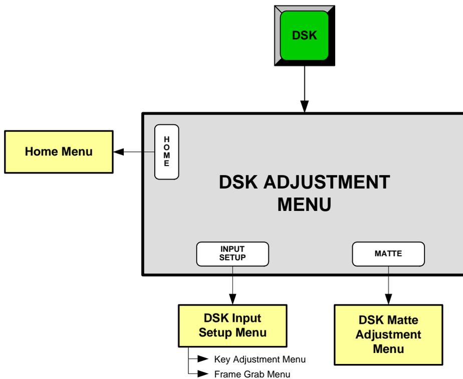
**Figure 4-47.** DSK Adjustment Menu Tree
