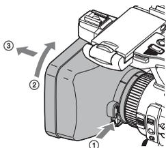
When attaching the optional wide-conversion lens, use the lens hood supplied with the wide-conversion lens.
