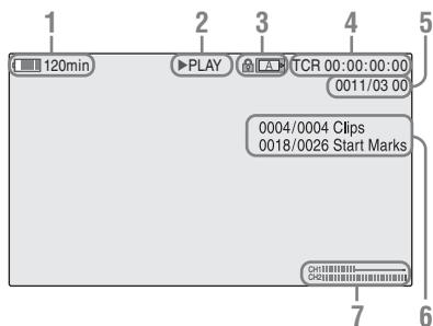
**1. Battery remaining/DC IN voltage**
