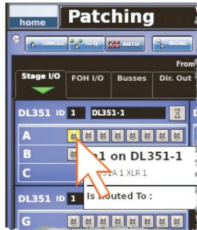
3. Select the destination patch connector. For example, in the **Inputs** tab of the **To** section, click the patch connector for input channel 14 (Mic14). It will now be patched to the source. If the new patch is carrying a signal, this audio may be heard, depending on the settings of the control centre.
