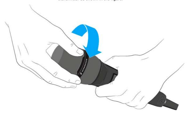
With some microphone modules, the upper part of the microphone basket can be screwed off. Ensure that you always completely unscrew the microphone module.
