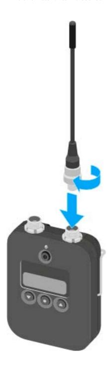
The antenna can be connected to the antenna socket very gently in only one direction. Do not use force to connect the antenna to the bodypack transmitter antenna socket.
