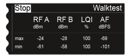
During the walk test, the Stop option in the top left of the display is high-lighted as the selection.
