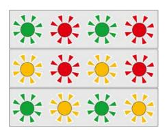
Flashing green/red >> rechargeable battery not inserted.
