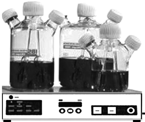
Fig. 2.3. Spinner flasks for suspension cultures. Cell cultures (suspension or monolayer) are started in T-flasks containing 25 ml medium. After reaching confluency the cells of two flasks are combined in a smaller (200 ml) spinner flask that is sitting in the CO 2 incubator. Cells in suspension are grown under constant stirring in 100 ml medium starting at \sim 10^5 ml/ml density. Logarithmic growth is maintained by scaling up daily from 100 to 200 ml medium, then switching to a larger spinner flask (2 l) and doubling the volume of the medium to 400, 800, and if necessary 1,600 ml. Up to 3\text{--}4 \times 10^8 cells can be grown in 1 week before starting elutriation.
