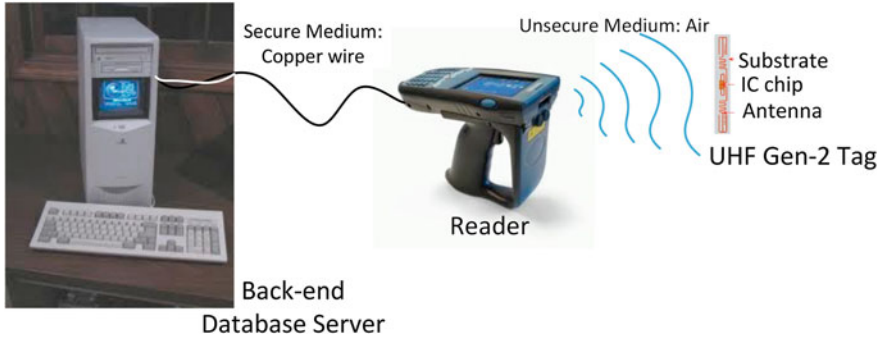
Fig. 1. A typical UHF RFID tag reading scenario
