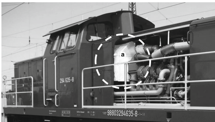
Fig. 2.20 Shunting locomotive from Deutsche Bahn AG with a combined DPF + SCR installation (Picture MTU)
