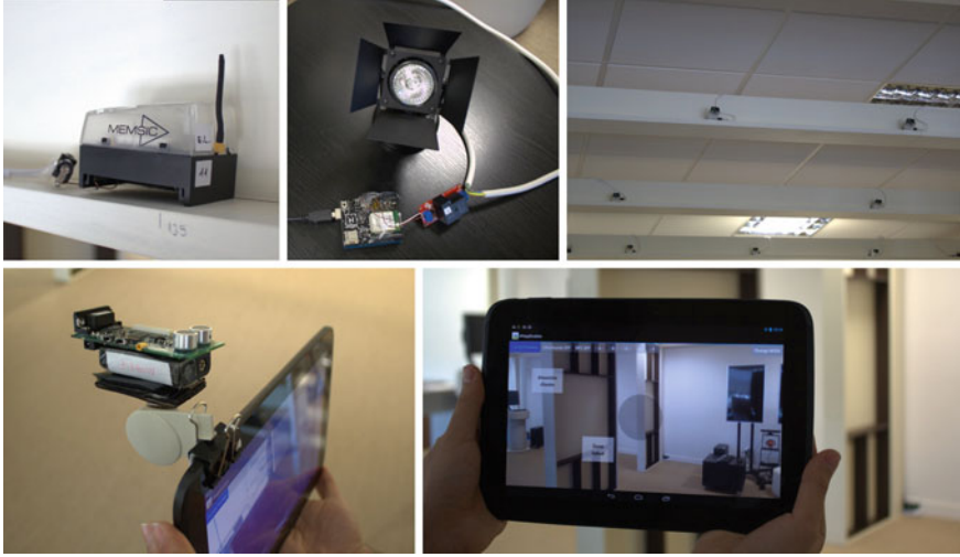
Fig. 9 Infrastructure deployed to simulate the Smart Shop. From top to bottom and right to left : a MicaZ node with a sensor board integrated, fixed to the ceiling; b Arduino Uno connected to a LED lamp; c Cricket-based network deployed strategically on a ceiling structure; d Cricket node attached to a tablet PC; e A tablet PC running an AR application
