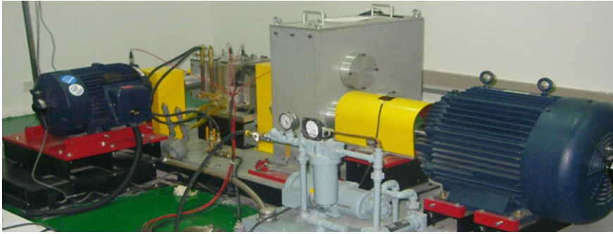
Fig. 2 Helicopter transmission system fault simulation platform
