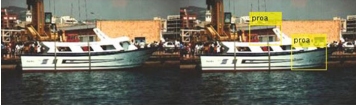
Fig. 3. Identification of vessel bow through HOG process
