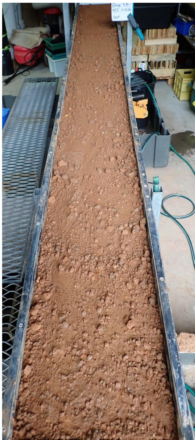
Figure 3: Eloise TD5 Material at (a) start (left) and (b) completion (right) of 5% slope flume run
