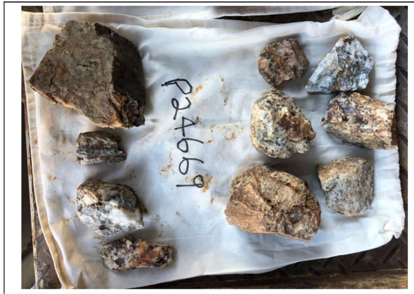
Figure 10: Sample P24669 grading 10.65g/t Au, 1.98% Cu & 158g/t Ag
