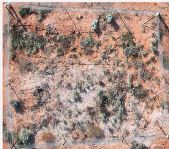
Figure 2: An example exploration drillhole that has been hydroseeded and fenced. The white coating on the soil is dried paper mache & native seed mix; providing structural stability, preventing erosion and holding the seed in place until germination occurs.
