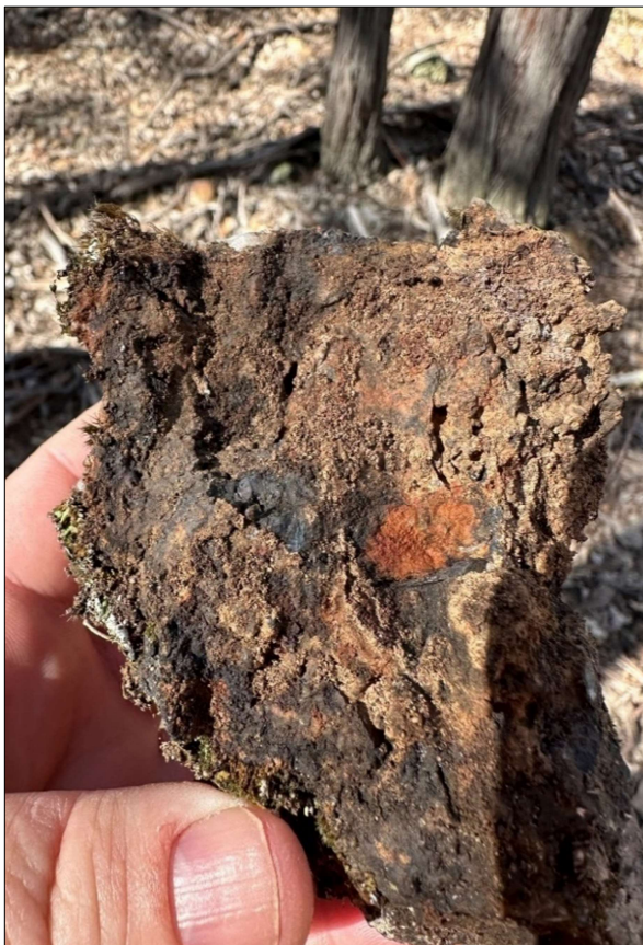
Figure 8 – Silver-Base metal mineralisation within ferruginous gossan yielding 87.8 g/t Ag, 1.5% Cu-Pb-Zn & >1% Ba from sample 3000728
