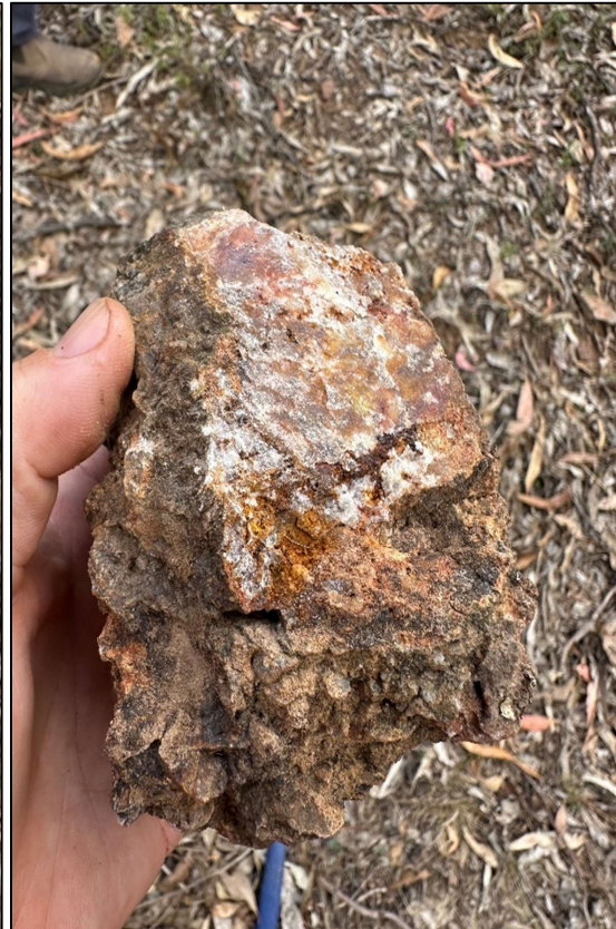
Figure 14 – Silver mineralisation within ferruginous quartz yielding 183 g/t Ag, 970 ppm Ba from sample 3000551
