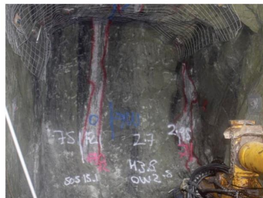
1085 Main Lode North - Cut 21 (Split fired cut)
