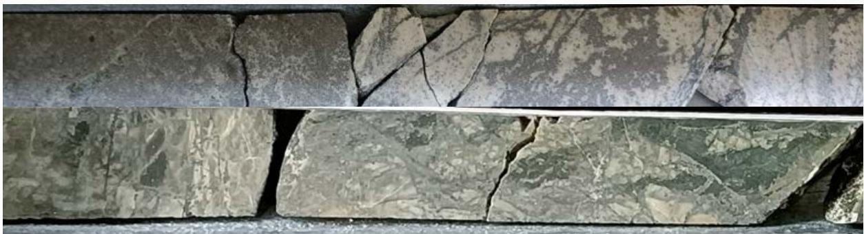
Figure 8 | Mineralised veins in Okvau diamond core. Hydrothermal Quartz Breccia with Arsenopyrite sulphides (interpreted feeder zone). Top photo: 78.30g/t Au from 158m (RCDD25OKV765). Bottom photo: 31.00g/t Au from 212m (RCDD25OKV712)
