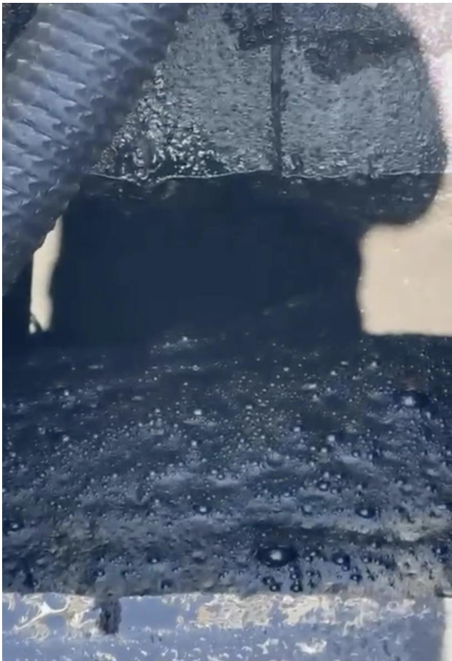
Figure 1: Photo of visible gas observed in drilling mud returns from Production Well One and evident along the length of targeted seam IIIb
