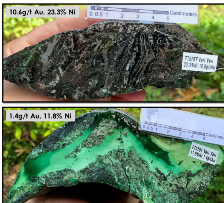
Plate1: Veri Veri creek float samples include massive nickel sulphide minerals (heazlewoodite, millerite, pentlandite) and nickel-bearing silicates including serpentinite and garnierite. Photo Right: boulder in creek from which grab sample top left was taken 10 .
