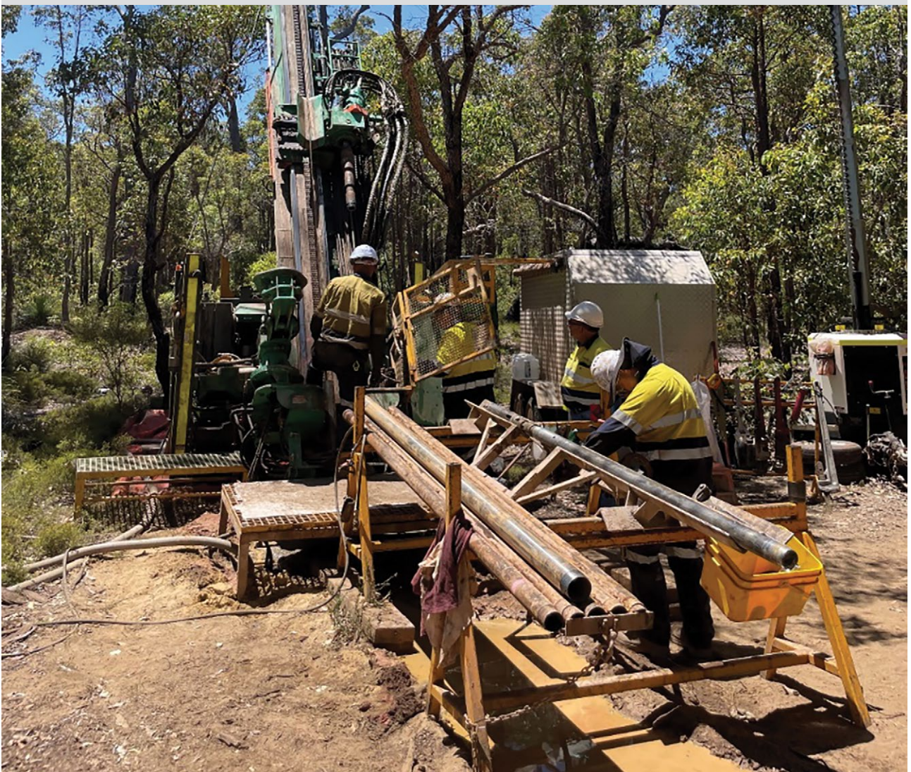
Figure 6: Diamond drilling underway at Greenbushes
