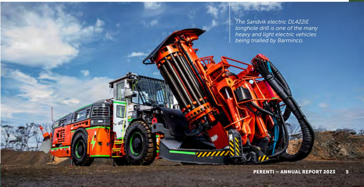
*The Sandvik electric DL422iE longhole drill is one of the many heavy and light electric vehicles being trialled by Barminco.*
