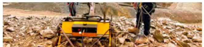
HALO is a robot that uses virtual reality technology to conduct safer rock scaling operations. The result of a two-year collaboration between Ausdrill, the University of Technology Sydney and the Innovative Manufacturing Cooperative Research Centre. HALO allows operators to use headsets and 3D virtual reality technology to scale walls, keeping them a safe distance away from rock scaling operations and out of the line of fire.
