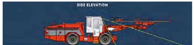
Currently operators rely on team members to ensure they are keeping a safe distance away from large equipment and out of the line of fire. The Jumbo Area Denial System automates this process by detecting reflective material, including people, in close proximity to development drills and automatically stopping the hydraulic functions of the drill booms once a reflection is detected. This system is currently in use at two sites, with further rollouts planned in FY24.
