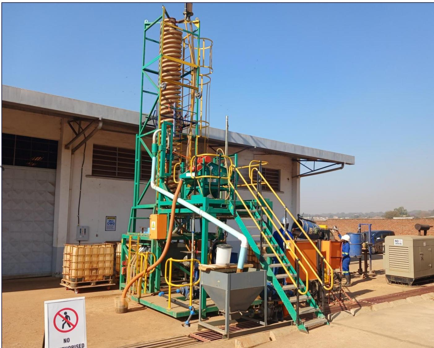
Figure 2: Spiral Plant installed at Sovereign's Lilongwe facility
