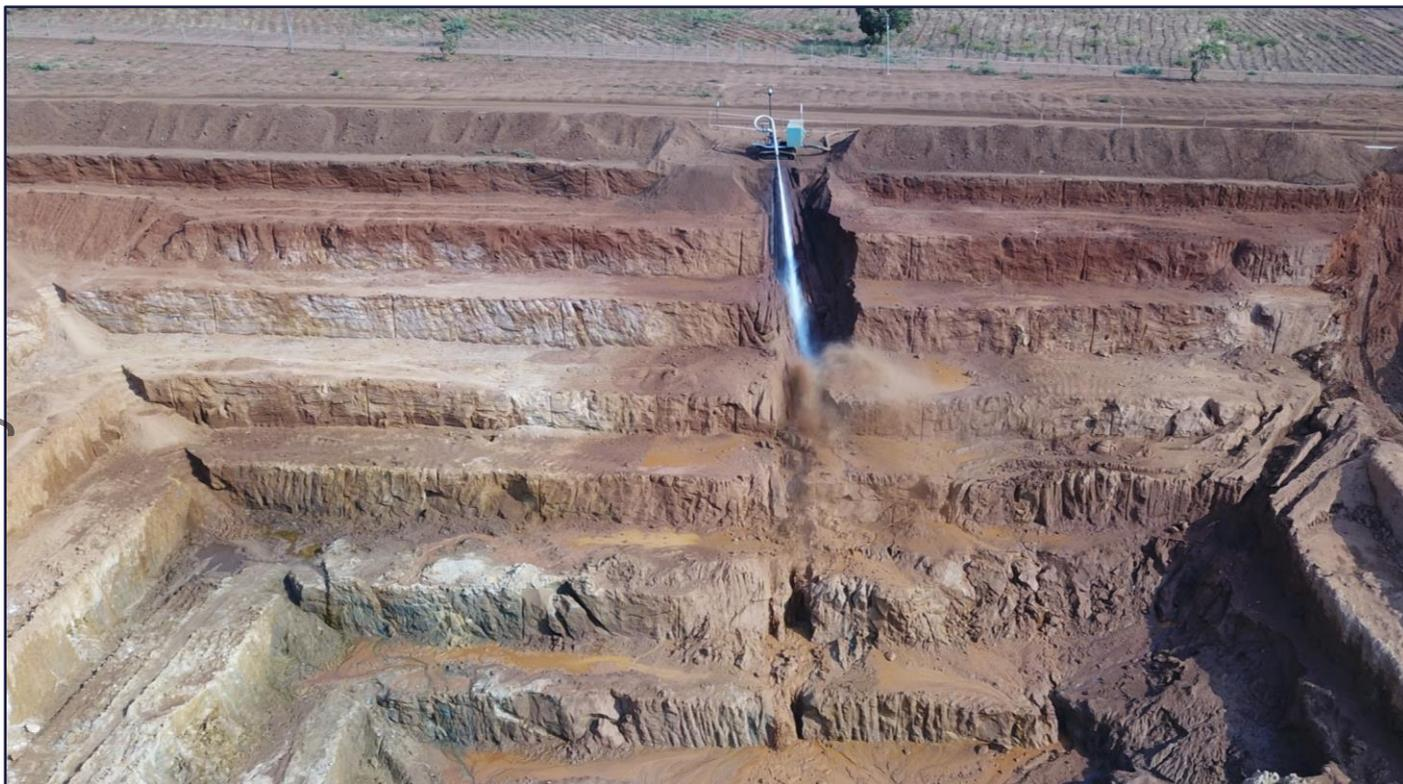
Figure 5: Hydraulic mined material (slurry) flowing freely to the collection point in the bottom of the sump
