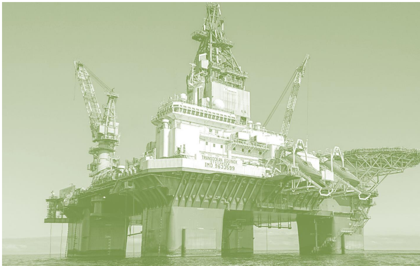
Figure 1: Transocean Equinox semi-submersible drilling rig
