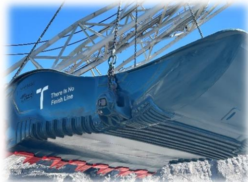
Refurbished High Performance Dragline Bucket
