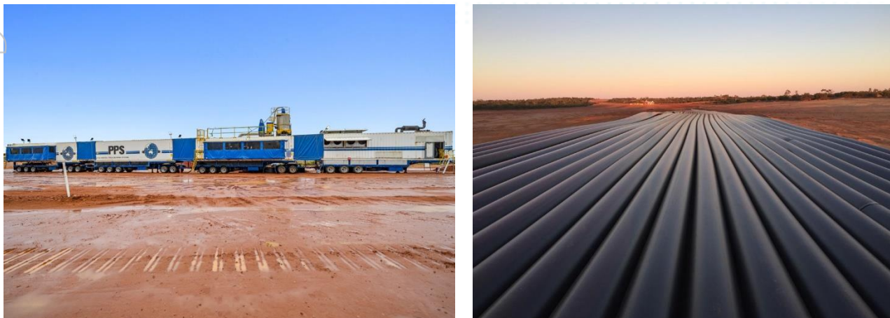
Figure 2 Polyline Pipe Systems pipe extrusion for the raw water borefield
