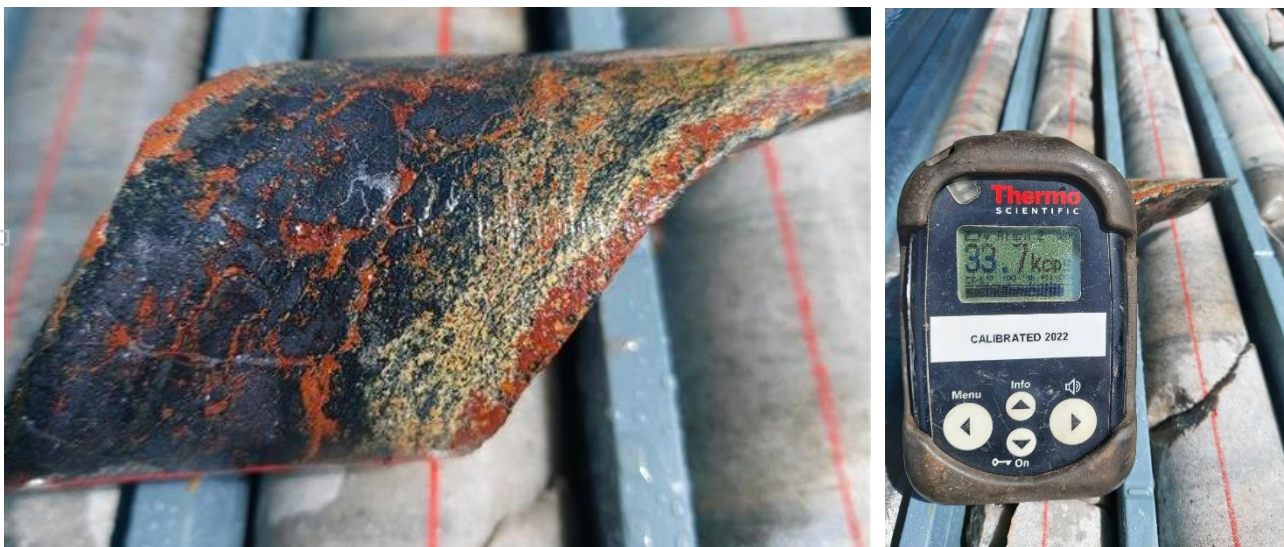
Figure 4: Very high-grade uranium vein in ARDD0006 (219m)
