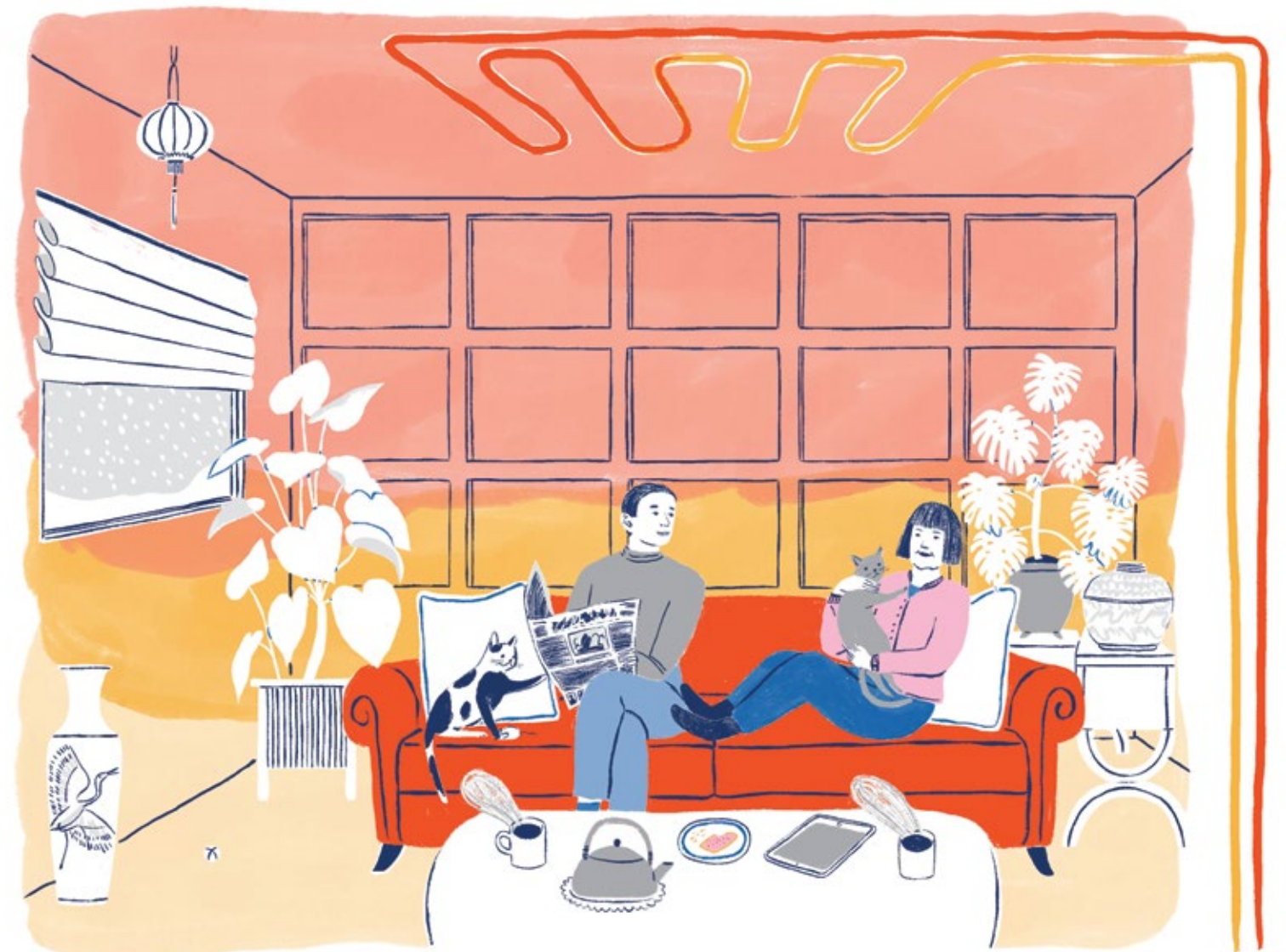
Building loops would heat and cool residential and commercial spaces by circulating through radiant ceiling panels.
