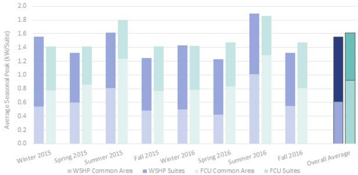
Figure 35: Building Level Peak - Breakdown of Common Area vs Suites
