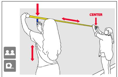
Using the measurement taken from the end of the raceway to the power hole, and the previously established edge, locate and mark the location of the power hole.
