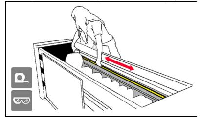
Place a piece of easily removable tape onto the wall at the center location of the raceway. From this point measure over until the edge of the raceway, where another piece of tape should be placed.
