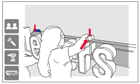
With your helper holding the other end, make connections between any adjoining raceways and slide the ends together.
